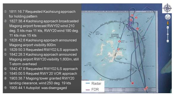
Figure 1.11-8 Superimposed GE222 flight path and VOR chart
