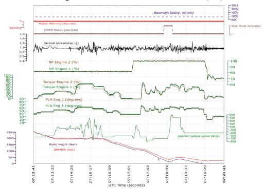
Figure 1.11-6 GE220 flight data plot (below 2,500 feet)
