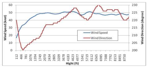
Figure 1.7-7 Wind profile from the surface to 9,000 feet
