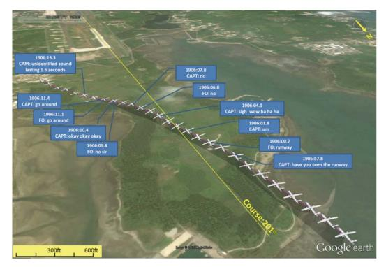
Figure 2.2-2 Aircraft track and altitude deviations as flight crew attempted to visually locate the runway.
