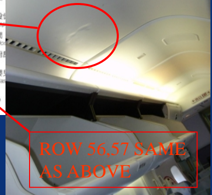
ROW 53,54 CEILING LATCH BROKEN & PNL DENT
