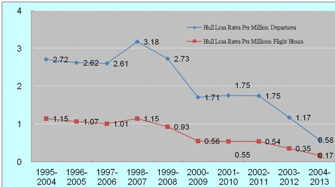
Figure16 : 10-year moving averages hull loss occurrence rates of Taiwan commercial jet airplanes
