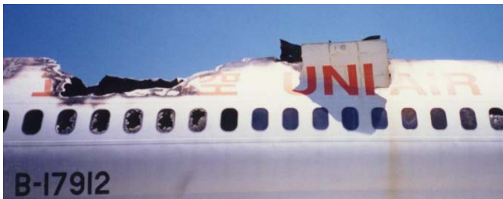
Fig. 1.12-4 The ripped-off cover
