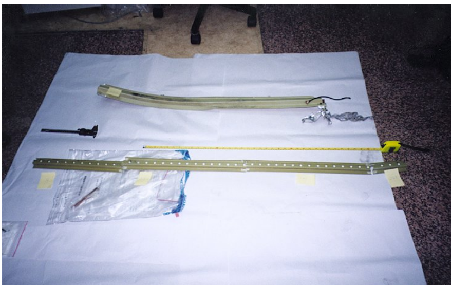
Fig. 1.12-9 Fragments of longitudinal beam and bin rail tie rod found on the runway (showing no burn signs)
