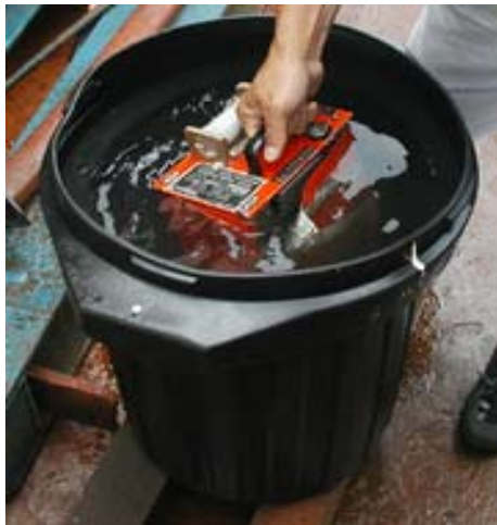
Figure 1.18-12 (a) An investigator was putting the CVR into fresh water- left photo, (b) Navy's diving bell was leaving the ocean surface with the FDR - right photo
