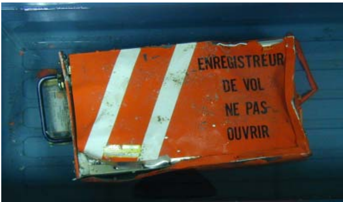
Figure 1.11-1 Damaged CVR in the cooler
