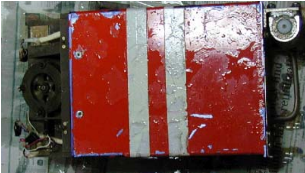
Figure 1.11-2 Damaged FDR in the cooler
