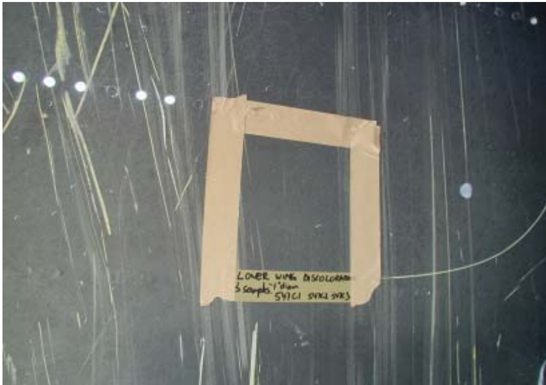
Figure 1.16-165 Discoloration sample 547 before cutting, showing the location from which samples 547C1, 547C2 and 547C3 were taken.
