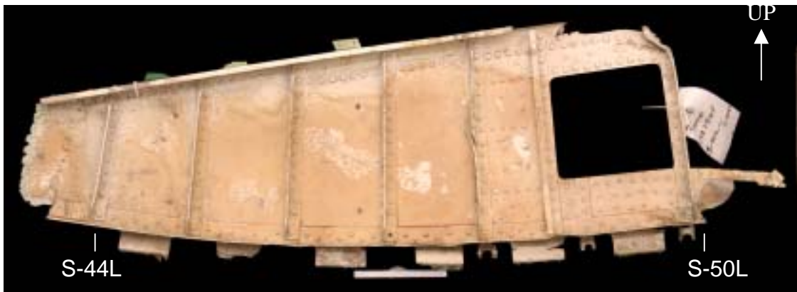
Figure 1.16-123 As received condition of the STA 1940 frame segment submitted for examination. The aft surface is shown in this view.
