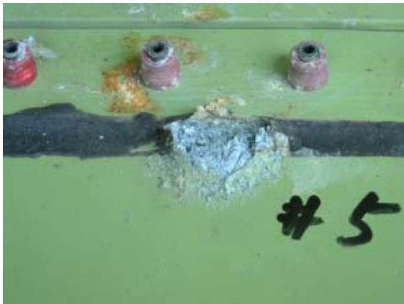
Figure 1.16-138 Higher magnification of #5 corrosion pit, before cleaning (1.46X)
