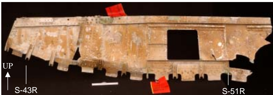
Figure 1.16-119 As received condition of the STA 2040 frame segment submitted for examination. The forward surface is shown in this view.
