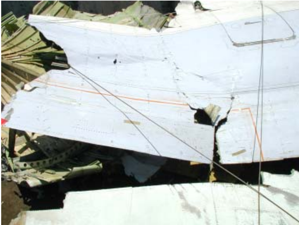
Figure 1.16-36 Item 640C1 and C2 Skin panel segments prior to removal from the parent item 640 wreckage in Makung, Taiwan.
