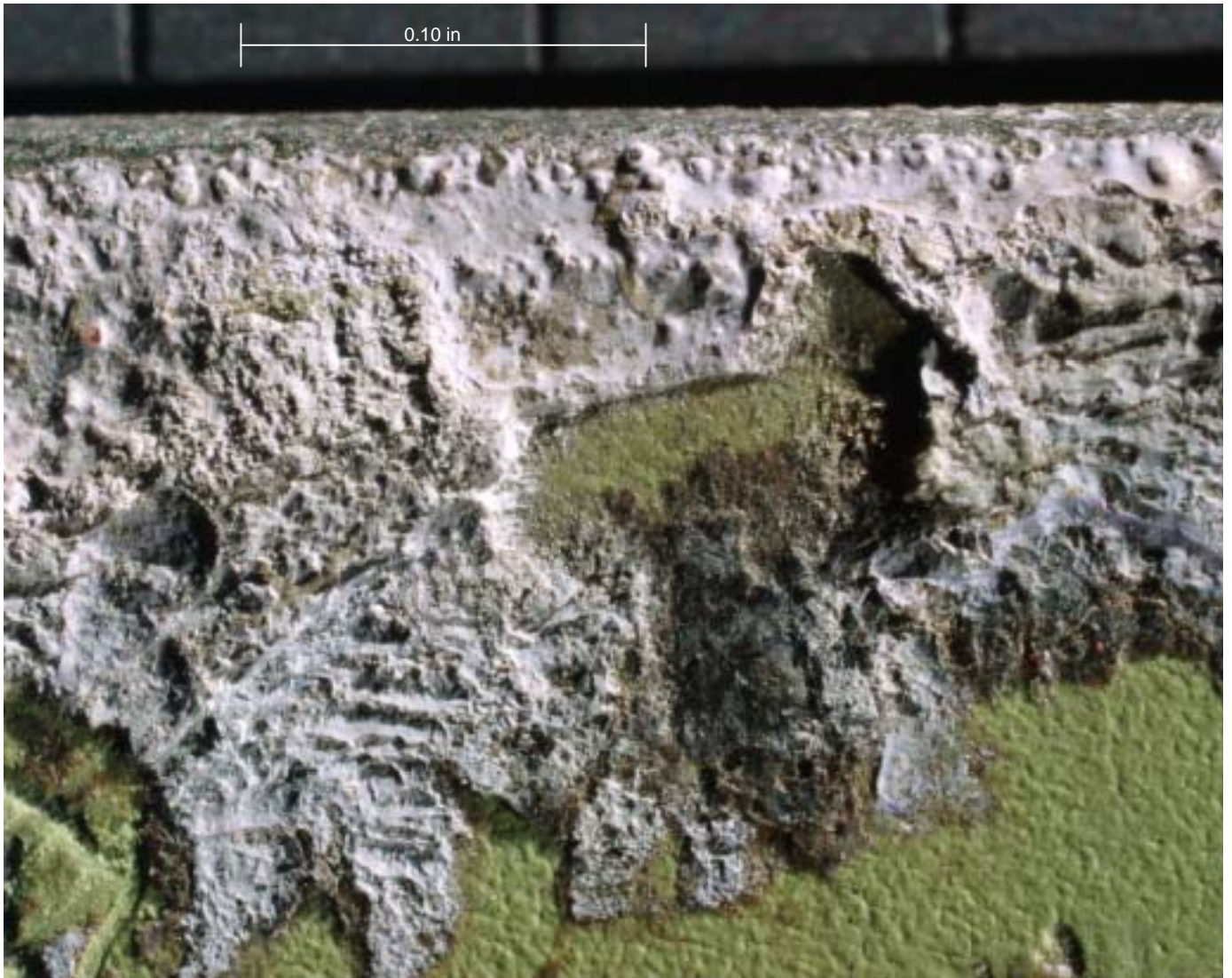
Figure 1.16-100 Higher magnification image of light colored deposit on faying surface of doubler in the vicinity of hole 15. Note the smooth bubbled appearance of the deposit adjacent to the edge of the doubler.
