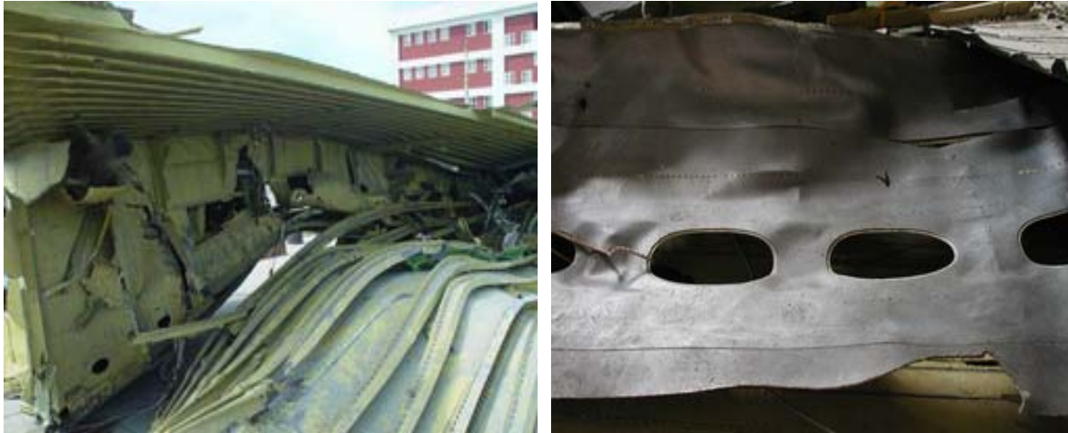
Figure 1.12-7 (b) Lower panel and midspar deformation on Item 547, (c) Localized deformation on outboard end of item 547
