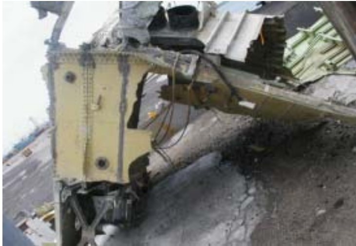
Figure 1.12-23 (b) Rear Spar Item #910 as recovered with segments connected
