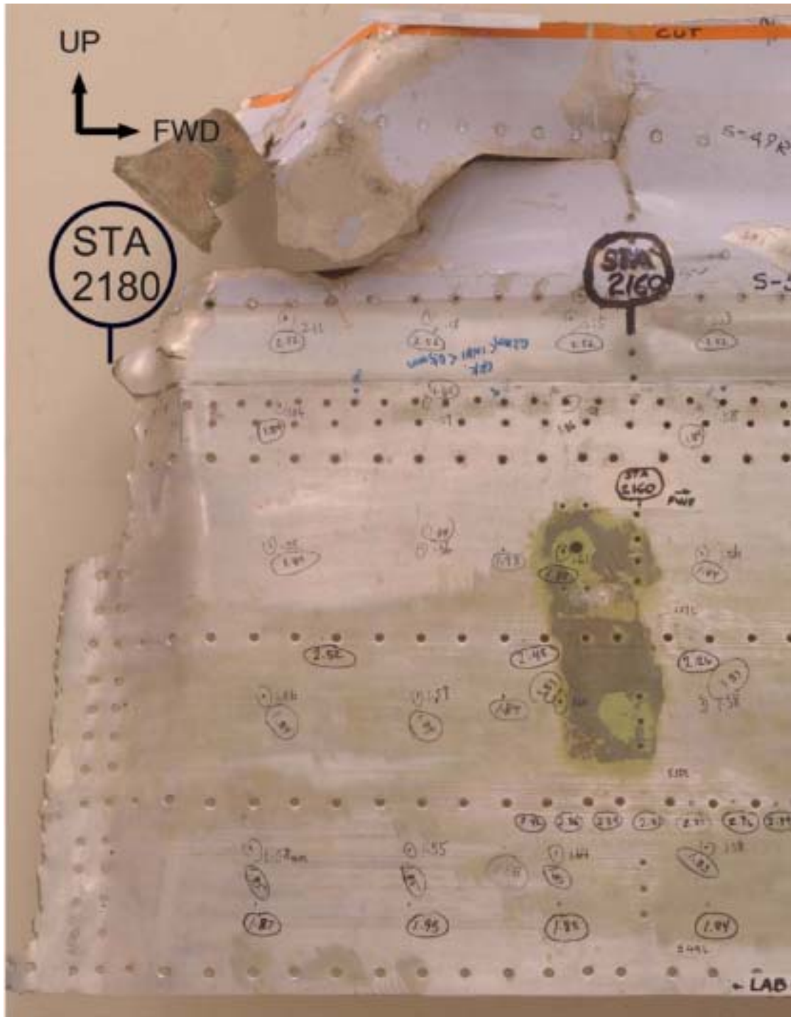
Figure 1.16-75 Skin thickness measurements- All measurements are in millimeters. Circled values were performed at Boeing
