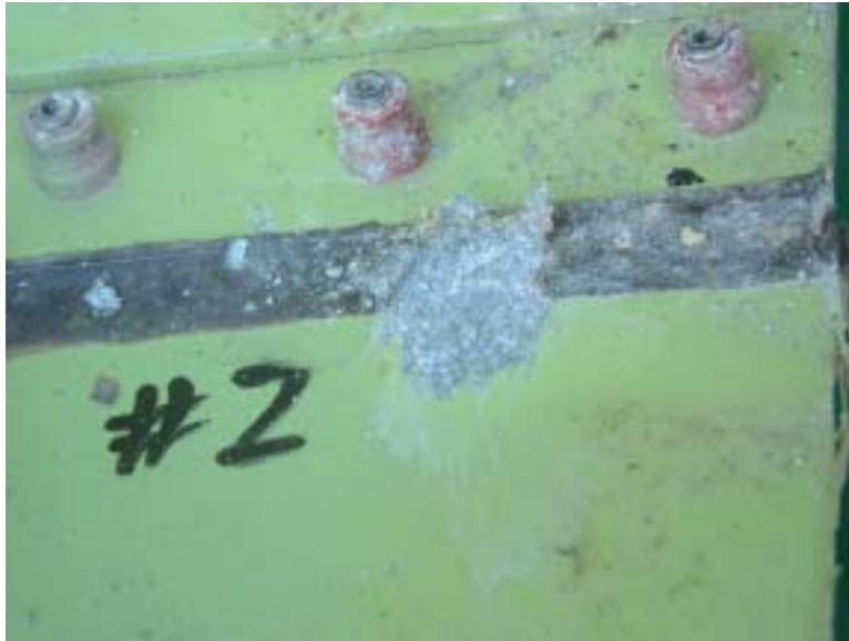
Figure 1.16-135 Higher magnification of #2 corrosion pit, before cleaning (1.52X)
