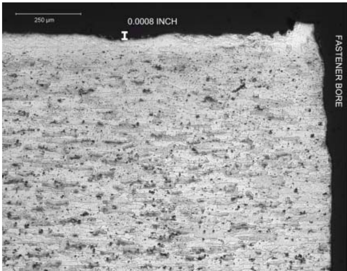
Figure 1.16-93 OUTER FASTENER ROW SCRATCH FEATURES AT PLANE A-A – Skin damage at this location was much less severe than on the left hand side of repair doubler. Skin cladding was not compromised by surface damage in this view.
