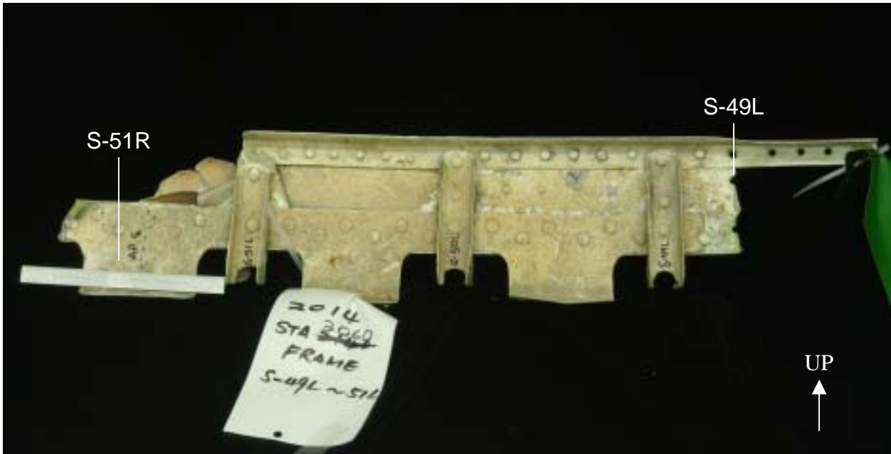
Figure 1.16-115 As received condition of the STA 2060 frame segment. The forward surface is shown in this view.
