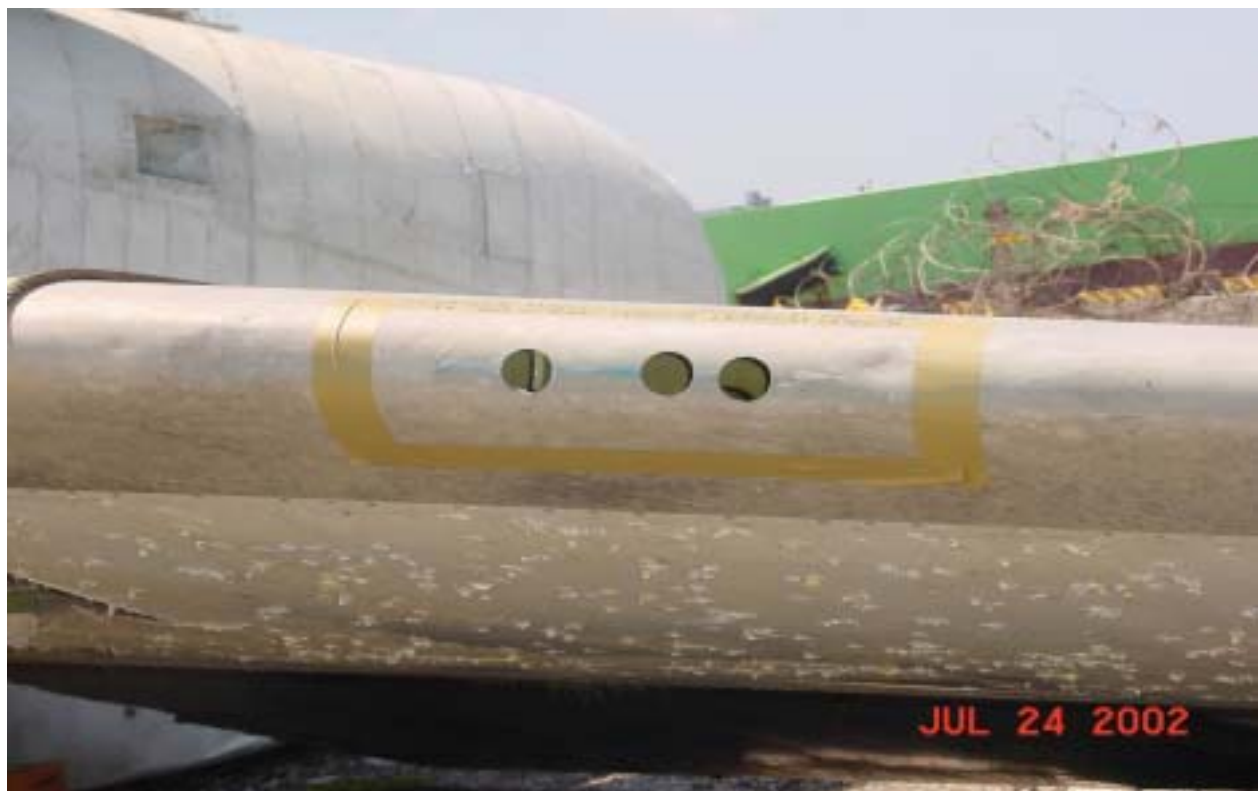
Figure 1.16-188 Photograph of the left horizontal stabilizer leading edge showing transfer marks on the applied coating.
