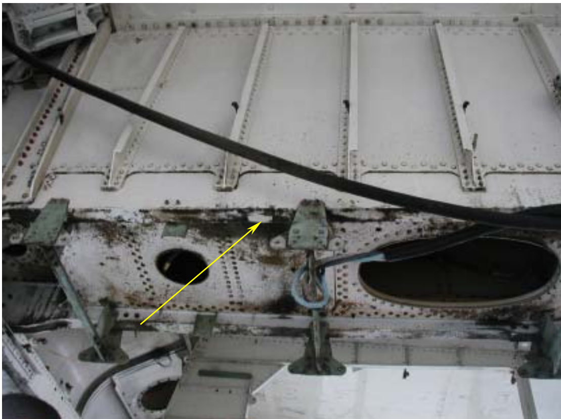
Figure 1.16-174 Photo showing location of reference discoloration sample from keel beam of retired 747.
