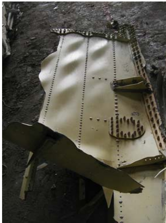
Figure 1.12-31 (a) Left S.O.B Rib Item #1264 showing web buckling
