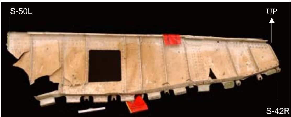
Figure 11.16-118 As received condition of the STA 2040 frame segment submitted for examination. The aft surface is shown.
