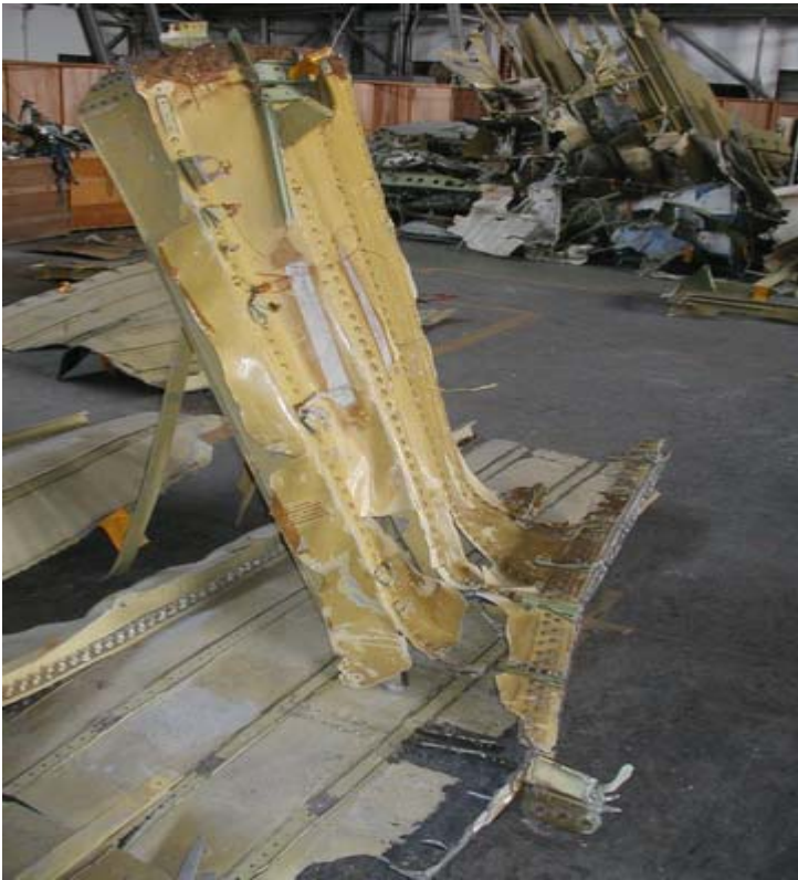
Figure 1.12-11 Front Spar Item 909 placed adjacent to Lower Skin
