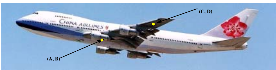
Figure 1.16-163 Photo of CI611 showing general locations from which discoloration samples were taken. Samples 642C3 and 547C3 were from wing center section as indicated by A and B. Samples 628C3 and 628C6 were from the right wing corresponding to the location indicated by C and D.
