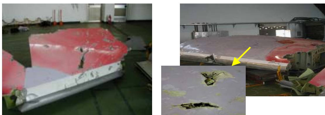
Figure 1.12-46 (a) Item 22- left photo, (b) Item 630C1 penetrations with 630C4 and 630C5 stringer segments placed- right photo
