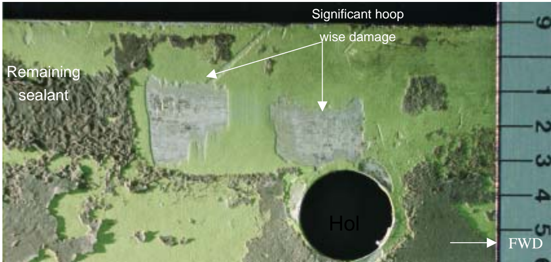
Figure 1.16-102 Faying surface of doubler in the vicinity of hole 6 showing an example of significant hoop wise damage at the 10:00 to 11:00 and 1:00 to 2:00 clock positions.
