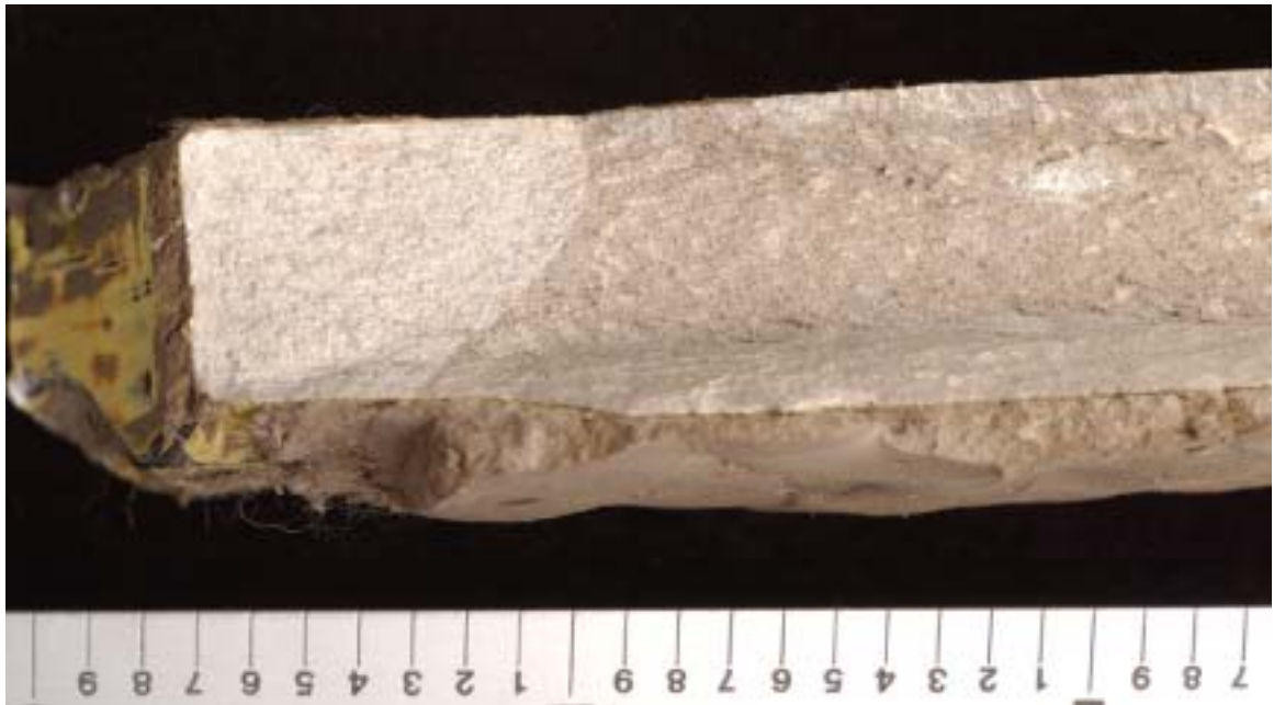
Figure 1.16-219 Photograph of the outboard half of the fracture of the upper tee fitting showing the distinct "thumbnail" region, associated with a flat profile.
