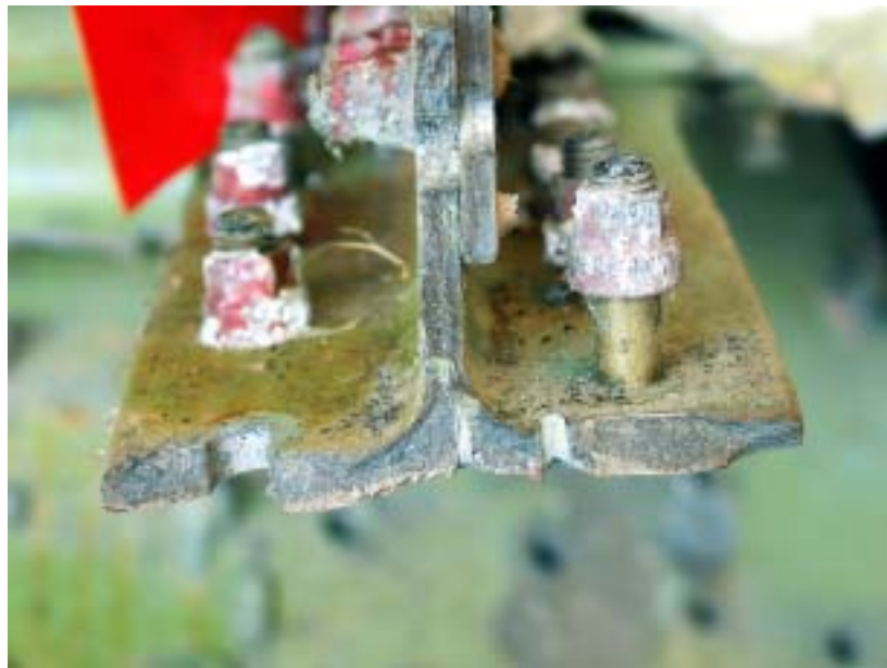
Figure 1.16-151 Macro fractographic examination of lower door reveal (1.53X)
