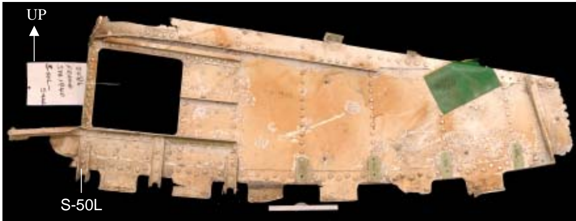
Figure 1.16-124 As received condition of STA 1940 frame segment submitted for examination. The forward surface is shown in this view.
