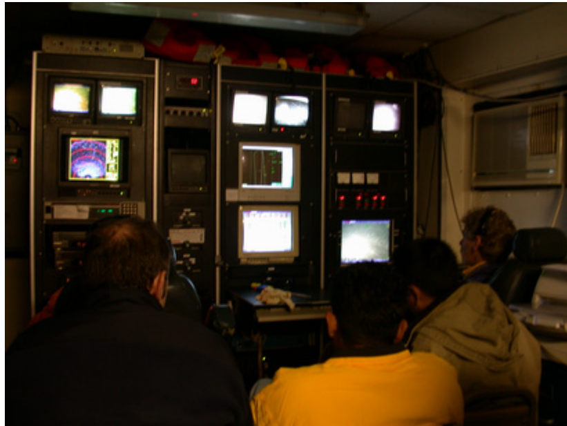
Figure 1.18-28 Visual check with ROV video camera and forward sonar scanning
