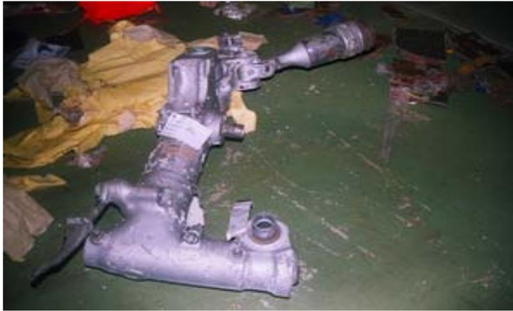
Figure 1.12-18 Landing gear shock strut
