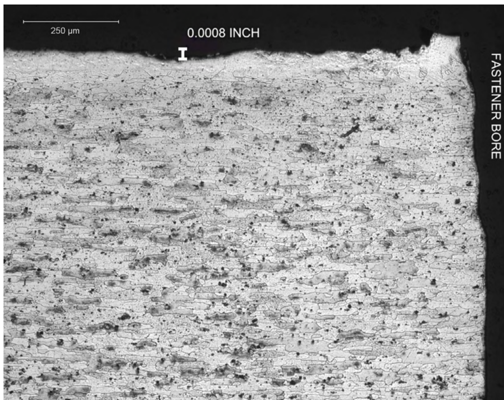
Figure 59. OUTER FASTENER ROW SCRATCH FEATURES AT PLANE A-A – Skin damage at this location was much less severe than on the left hand side of repair doubler. Skin cladding was not compromised by surface damage in this view.
