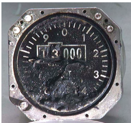
Figure 43: Cabin Altimeter Indicator, glass bezel removed
