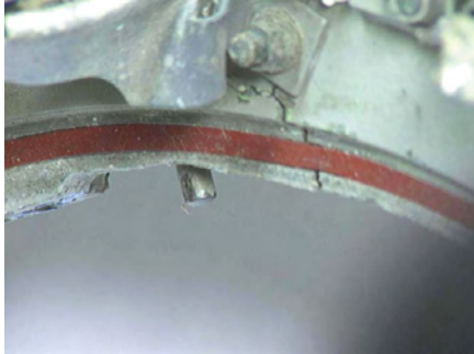
Figure 204: Exterior door open, forward/lower stop pin, HS P/N 730539-1, as viewed from inside.
