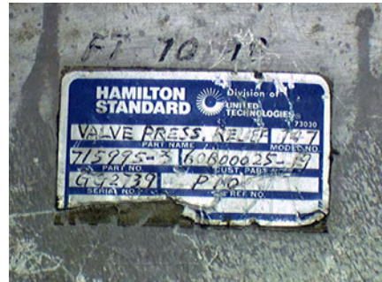
Figure 175: Lower Pressure Relief Valve, data plate identification.
