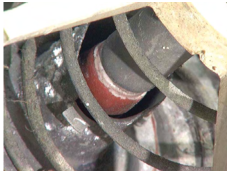
Figure 235: Center diaphragm, HS P/N 727401-1 appears to be intact and the bond portion can be seen; looks normal.
