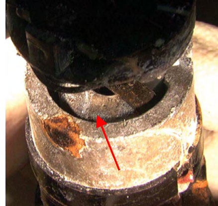
Figure 18: LEFT, OUTFLOW VALVES Position Indicator showing witness mark after moving armature.
