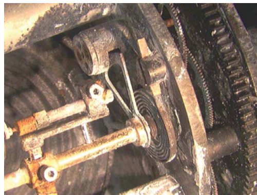
Figure 46: Cabin Altitude Indicator, bellows, visible damage
