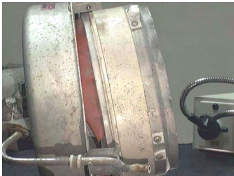
Figure 149: Offset angle between valve housing and gate.
