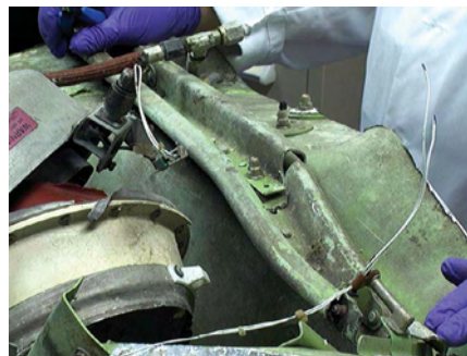
Figure 181: Lower Pressure Relief Valve. Cut switch lead wire B, step 2 in removal of lower valve (after cut).
