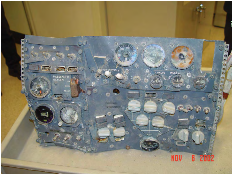
Figure 1 : Section of Flight Engineer's Panel
