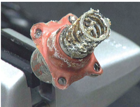
Figure 255: Integral sensor spring and diaphragm.
