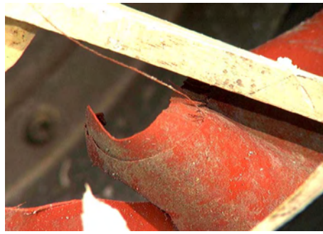
Figure 227 : Outer diaphragm HS P/N 727403-1, torn location.
