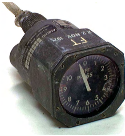
Figure 50: Cabin DIFF PRESS Indicator • Water stains inside glass face. • Needle is indicating below zero.
