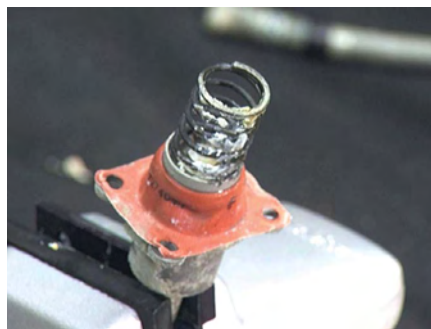
Figure 166: Diaphragm appears to be intact.
