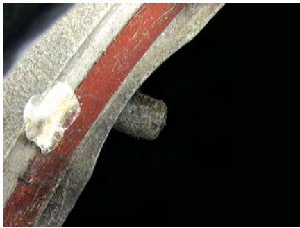
Figure 122 : Overview of aft/upper stop pin, as viewed from inside.
