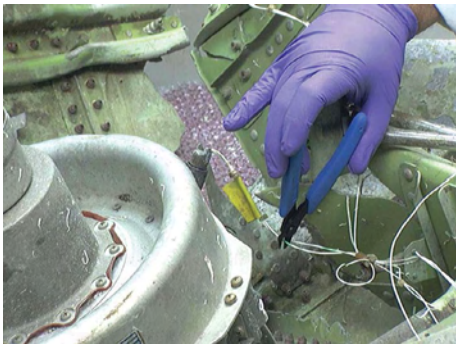
Figure 88: Prior to cutting switch lead wires.
