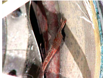
Figure 145: Diaphragm, 75 % of outer circumference is torn/split.
