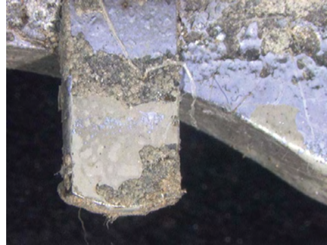
Figure 137: Aft/lower stop pin, close-up of figure #136. • Paint is chipped.
