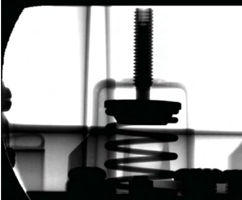
Figure 259 : Integral control adjustment spring.
