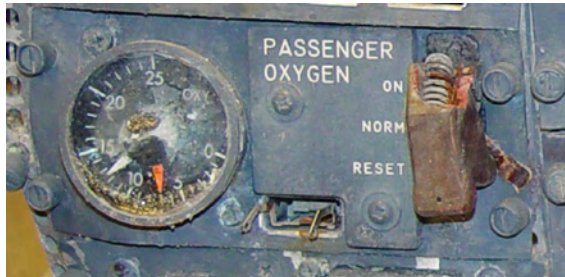
Figure 53: Passenger Oxygen Panel, module M183.
