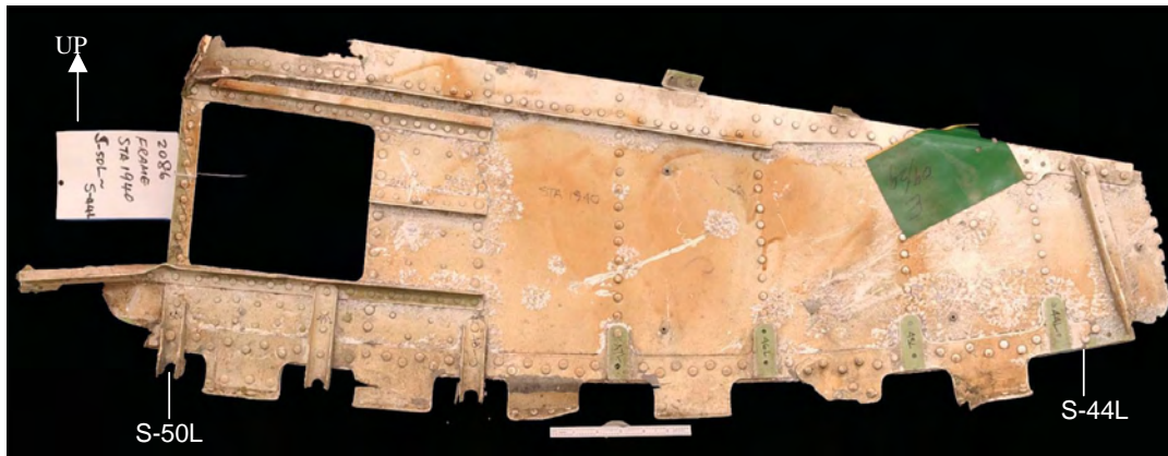
Figure 90. As received condition of STA 1940 frame segment submitted for examination. The forward surface is shown in this view.
