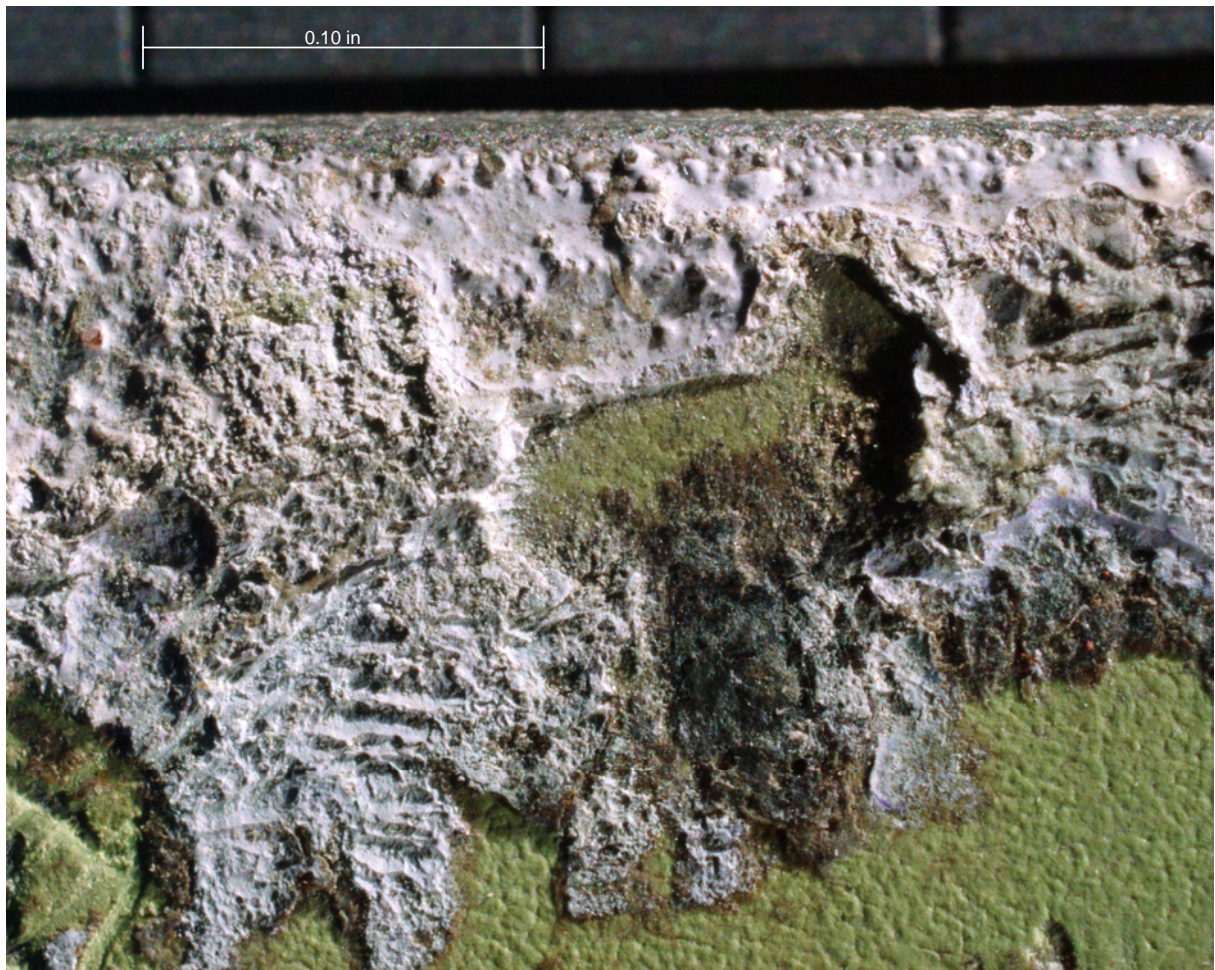
Figure 66. Higher magnification image of light colored deposit on faying surface of doubler in the vicinity of hole 15. Note the smooth bubbled appearance of the deposit adjacent to the edge of the doubler indicative of paint flow into the joint.
