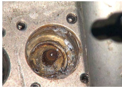
Figure 170: Integral ambient sensor poppet housing bore. • Poppet was free.
