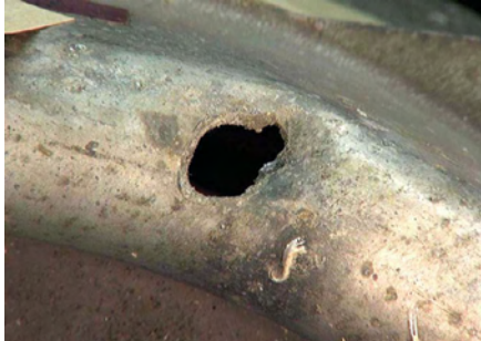
Figure 209: Hole penetrating support housing, HS P/N 727405-1. • Hole is approximately 0.365 inch x 0.560 inch.
