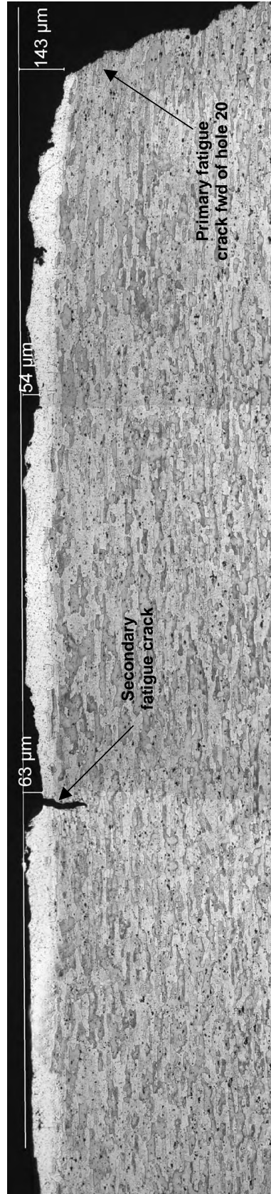
Figure 64. Metallographic montage through the area indicated in Figure 63 above. The line shown was projected back to an area of undisturbed clad material to determine the depth of the scratches at the primary and secondary fatigue cracks present in this area.
