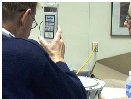
Figure 267: Comparison unit*, door A tension, 2.85 pounds (opening force from center edge of door).
