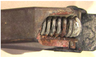
Figure 61: Top view of switch guard damage.
