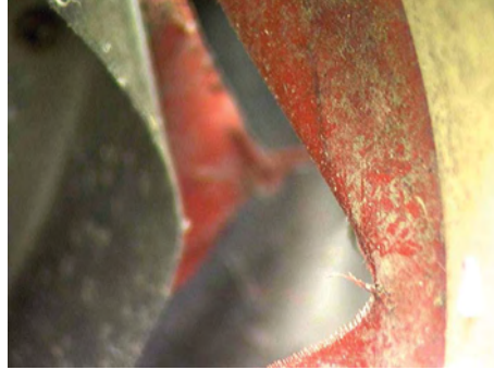
Figure 231: Outer diaphragm damage.
