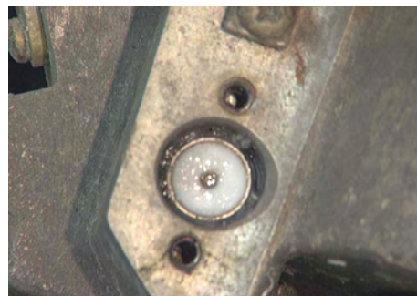
Figure 252: Remote ambient sensor, opposite end of poppet and guide.
