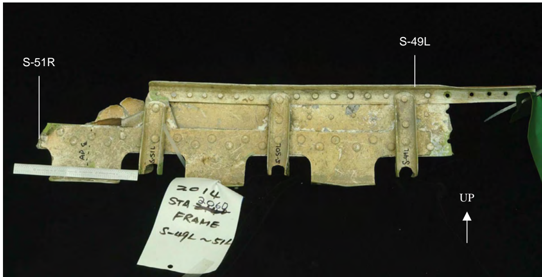
Figure 81. As received condition of the STA 2060 frame segment. The forward surface is shown in this view.
