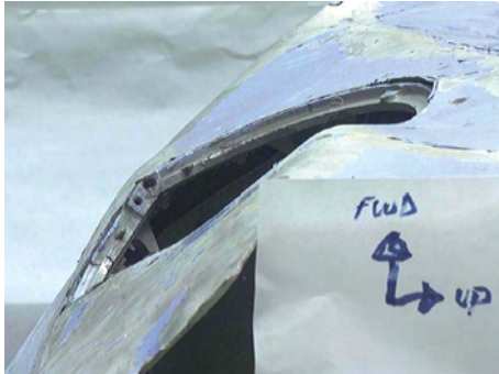
Figure 183: Skin distortion at valve mounting location.
