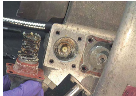
Figure 250: Showing remote ambient sensor removed.
