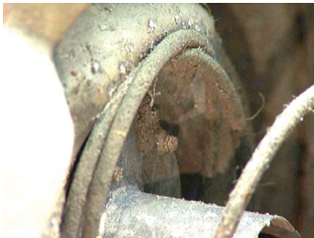
Figure 238: Gate return spring is over end showing intertwining of end coil and the active coil.
