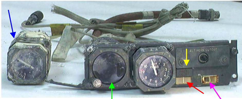
Figure 37: M188 panel. Note that the vertical speed indicator was detached from the module.
