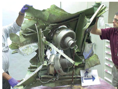
Figure 79: Upper & Lower Pressure Relief Valves, as installed, as viewed from inside.
