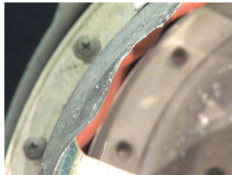
Figure 139: Close-up of knife-edge damage.
