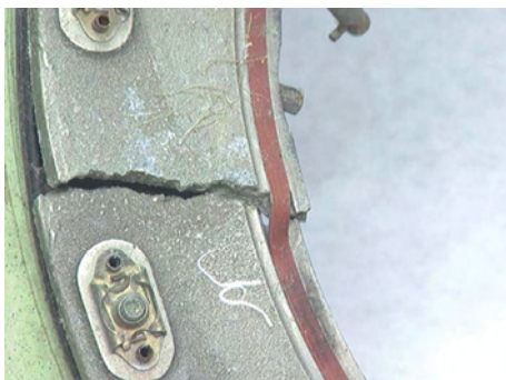
Figure 97: Non-metallic washer (gate seal) - continuous ring.
