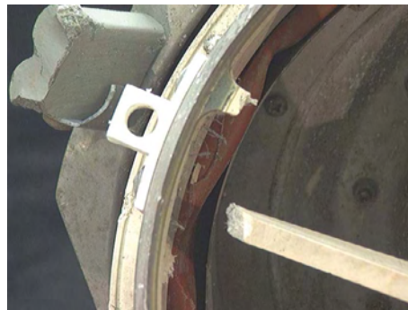
Figure 217: Broken web detail.
