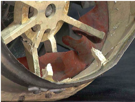
Figure 220 : Detail of more broken webs.
