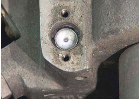
Figure 167: Remote ambient sensor poppet and guide, opposite side - relatively clean.
