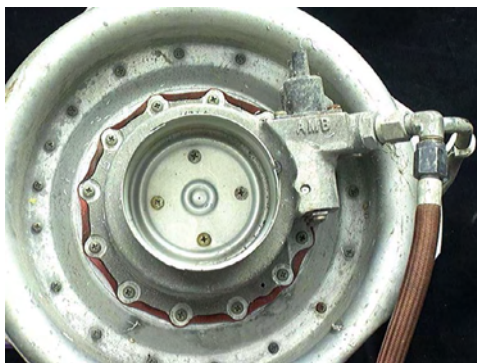
Figure 156: Overview of control and filter assemblies.
