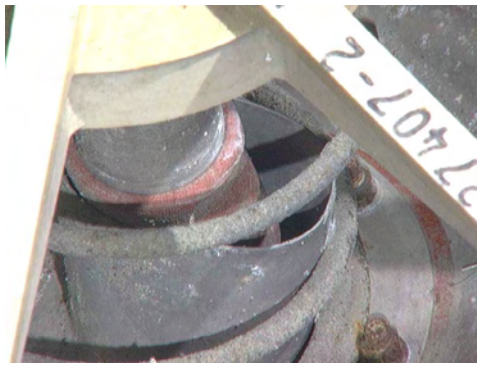
Figure 154: Center diaphragm guide, HS P/N 727411-1, showing distortion of guide itself.
