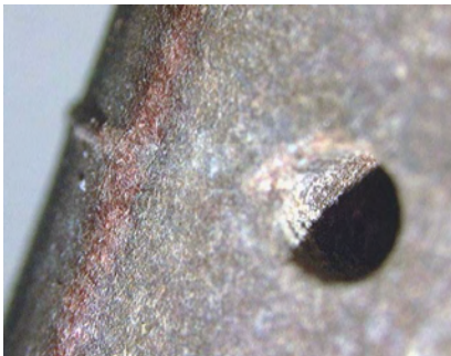
Figure 63: Switch guard safety wire (breakaway wire) hole (top view).
