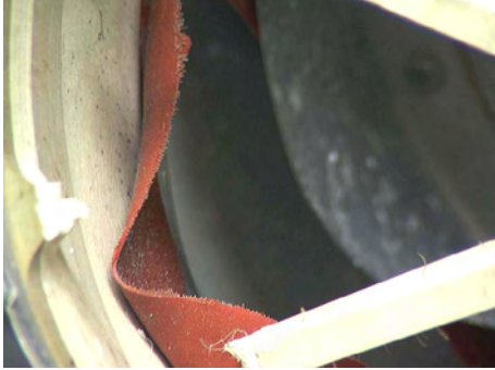
Figure 230: Outer diaphragm damage.
