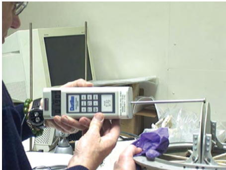
Figure 271: Comparison unit*, both doors open, closing one, 1.90 pounds (pulling at center of door).
