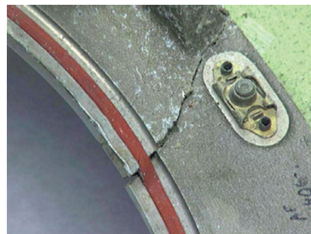
Figure 98: One slight cut adjacent to housing fracture.
