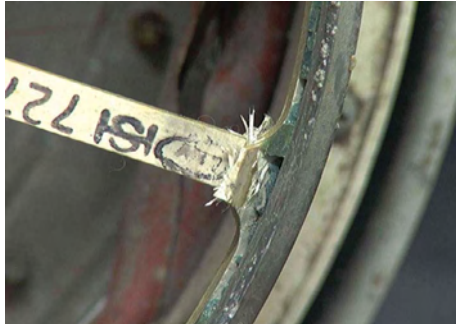
Figure 142: Overview, close-up of typical web fracture.
