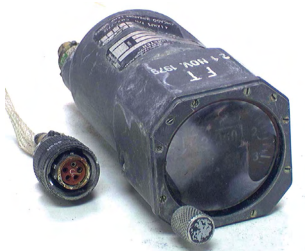
Figure 42: CABIN ALT Indicator (Ref. Figure 39, green arrow for location on module)
