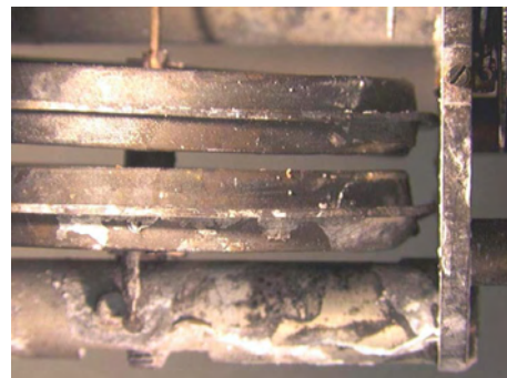
Figure 47: Cabin Altitude Indicator, bellows displacement
