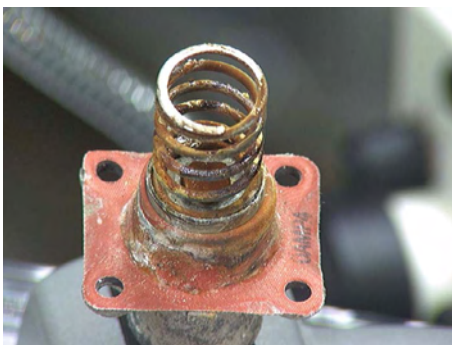
Figure 171: Integral ambient sensor spring & diaphragm. • Heavy hardened corrosion on spring and diaphragm in localized areas. • Corrosion on spring seat almost all the way around.
