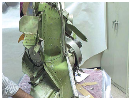
Figure 80: Frame, centerline (C/L) of stringer 31, looking fwd (frame view station 780).
