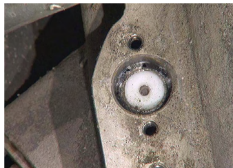
Figure 172: Opposite end of integral ambient sensor poppet and guide. • A little moisture is present.
