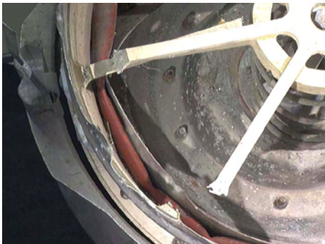
Figure 234: Outer diaphragm, intact (not torn) portion.
