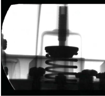
Figure 244: Integral sense control, adjustment spring.
