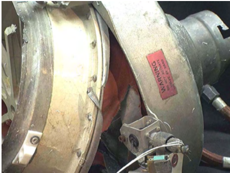
Figure 232: Side view of gate assembly & valve cover, showing the approximate 30° angle between gate assembly & valve cover.
