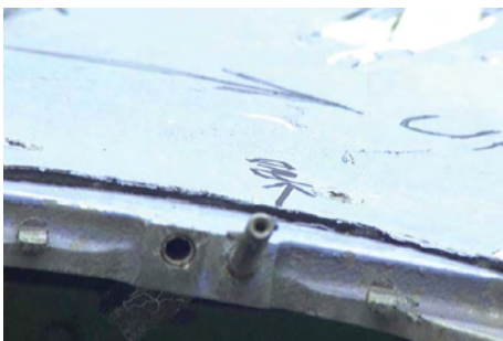
Figure 103: Forward/upper hinge pin, physically rotated by hand so that bent portion was oriented outboard.
