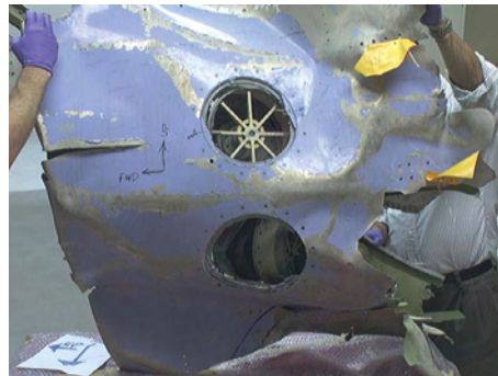
Figure 5: Pressure Relief Valves
