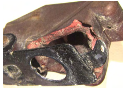
Figure 62: Bottom view of switch guard damage.
