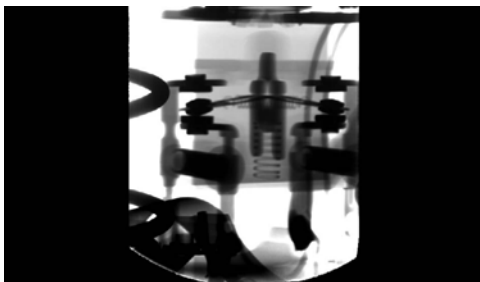
Figure 265: New switch, closed valve, not closed contacts.
