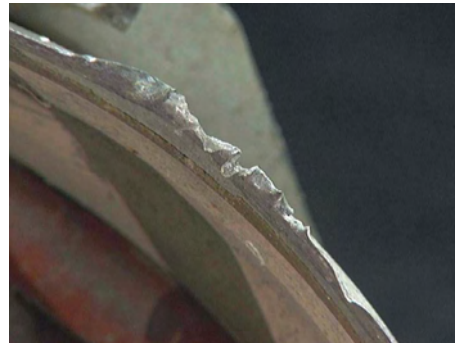
Figure 221 : Knife-edge close-up of damage.
