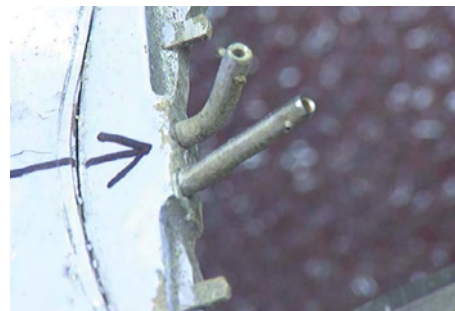
Figure 107: Aft hinge & stop pins, (looking from outside to inside) • Aft/upper hinge pin (lower pin in photo) is difficult to rotate. • Aft/lower hinge pin (upper pin in photo) rotates.
