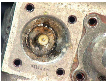
Figure 251: Close-up of salt deposits inside housing bore.
