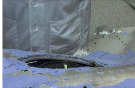
Figure 77: Upper pressure relief valve, (center of picture) distorted exterior skin.
