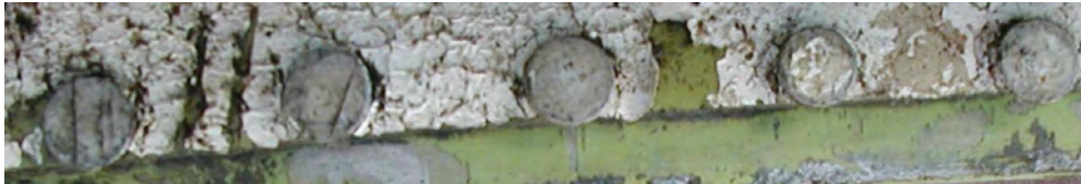
Multiple crack initiation sites along length
