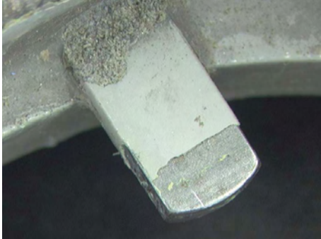
Figure 198: Forward/upper stop pin as viewed from outside looking inside.. • Pin is relatively straight.
