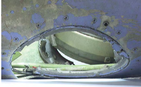
Figure 178: External view of opening for Lower Pressure Relief Valve, looking inside.
