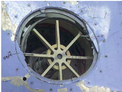
Figure 83: Upper Pressure Relief Valve, orientation as installed on airplane.
