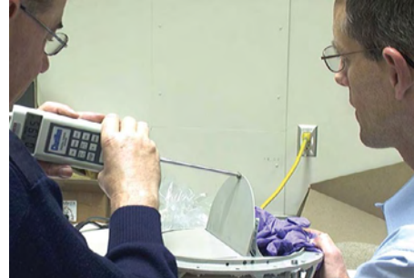
Figure 270: Comparison unit*, door B compression (closing), 1.95 pounds (push at center of door to close door).
