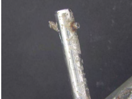
Figure 105: Detail of forward/upper hinge pin end.
