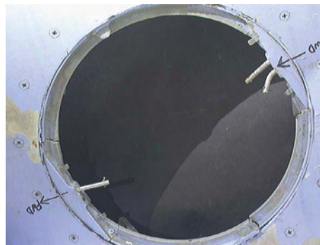
Figure 93: Upper Pressure Relief Valve, pins are in approximately "door closed" position.
