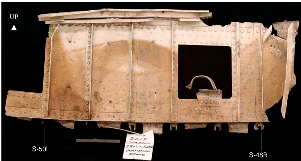
Figure 75. As received condition of the STA 2100 frame segment submitted for examination. The aft surface is shown in this view.
