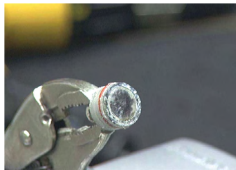
Figure 257: Plug for integral sensor, seal looks normal and uncut.
