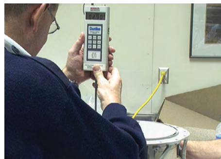
Figure 268: Comparison unit*, door B tension, 2.90 pounds (opening force from center edge of door).
