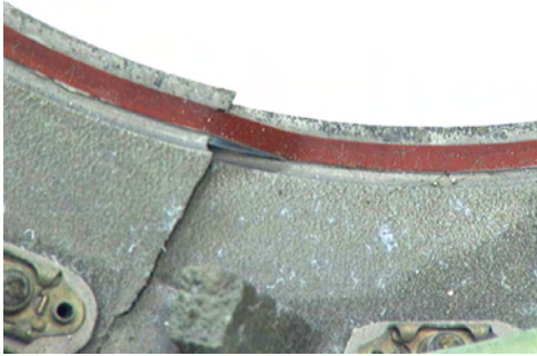
Figure 99: Another cut on the seal.
