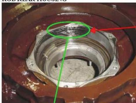
Deposits located on the inner diameter of the N° 15 Roller Bearing sleeve.
