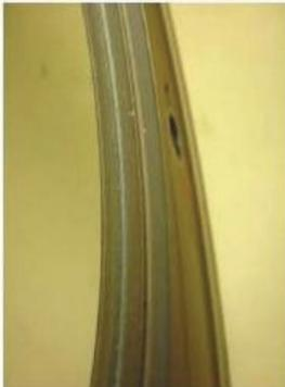
Loss of plasma coating on the air seal diameters.
