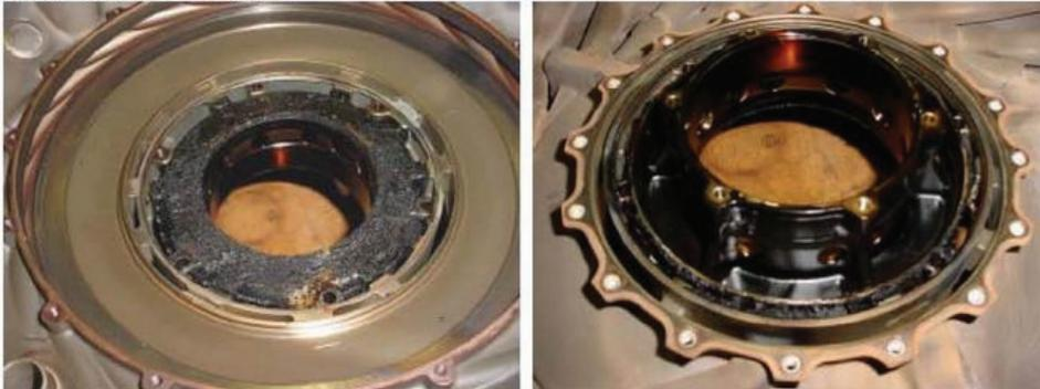
The front and rear surfaces of the N° 5 Bearing area are covered by coked oil deposits.
