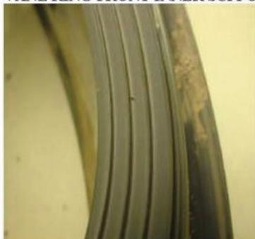
Loss of plasma coating on the air seal diameters.
