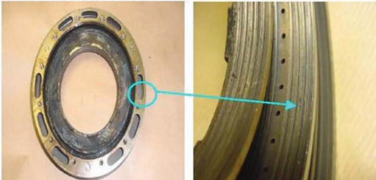
All the internal surfaces are covered by coked oil deposits.
