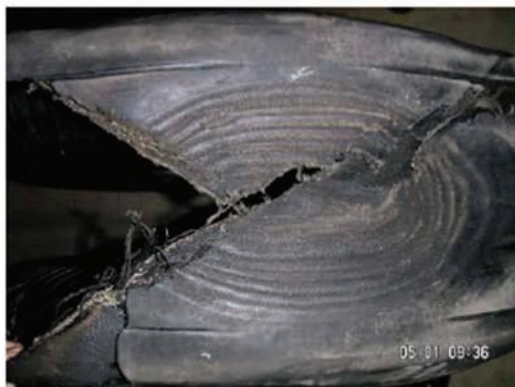
Photo 4: Flat spot along with a diagonal-break
