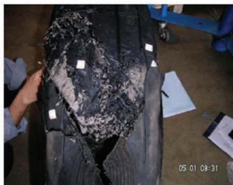
Photo 3: Reassemble the returned pieces on the casing
