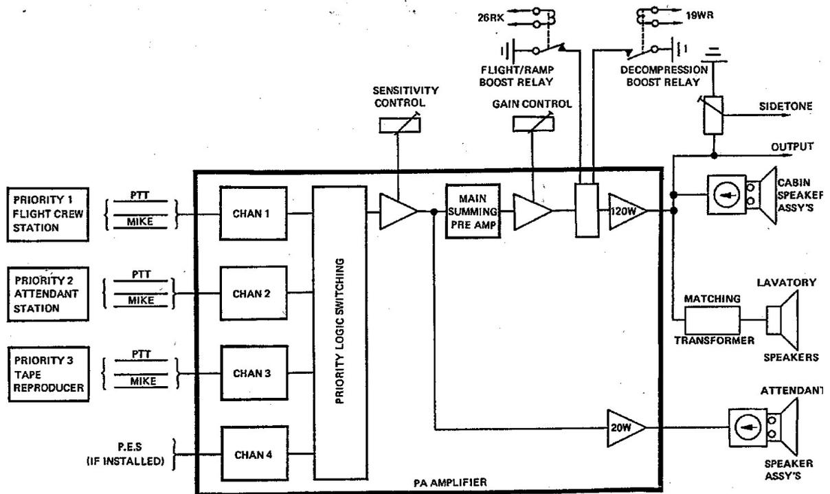
Figure 1.4-5 Priority Block Diagram
