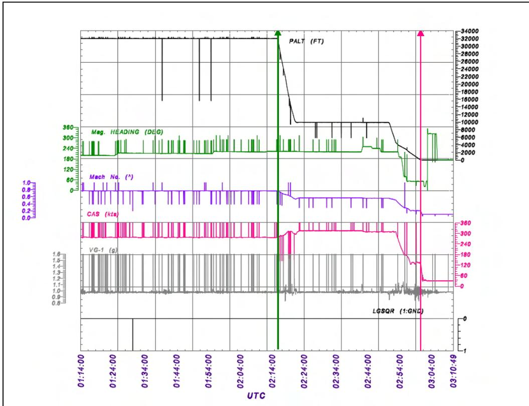
Fig. 1 KE691 relevant DFDR parameters plot (3,300ft ~ landing roll)
