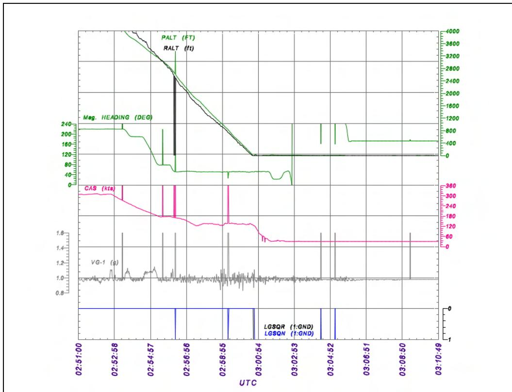
Fig. 2 KE691 relevant DFDR parameters plot (4,000ft ~ landing roll)
