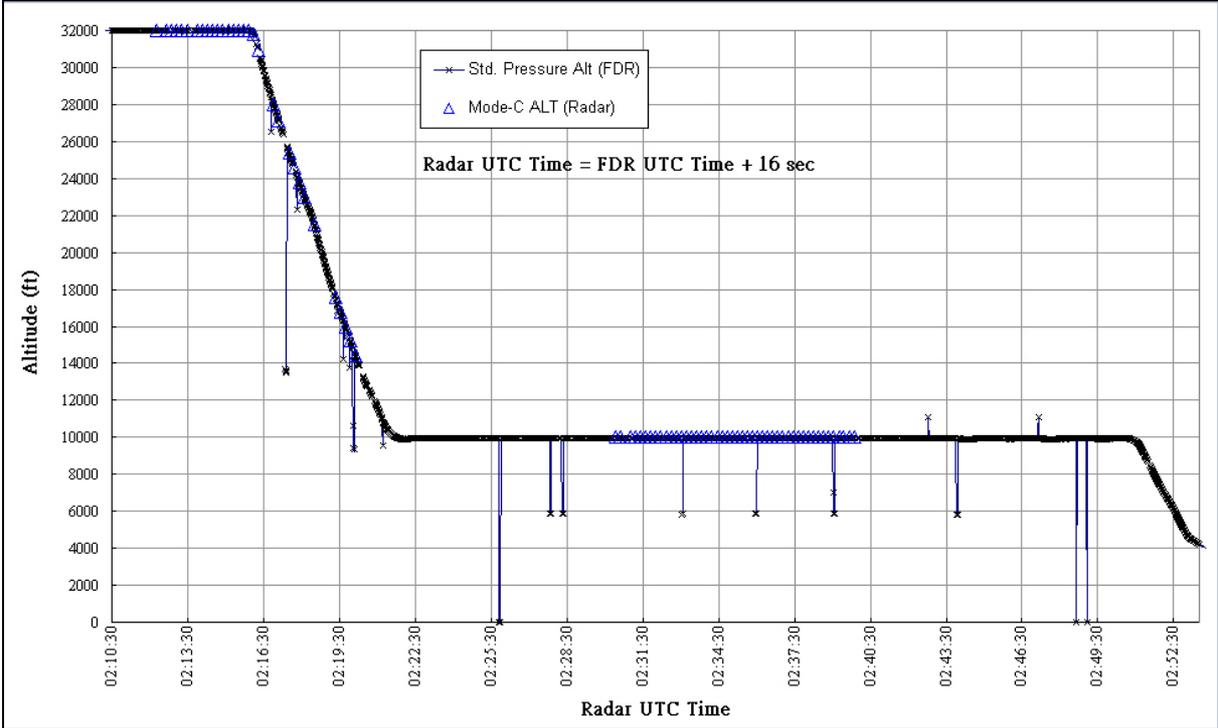
Fig. 3 KE691 relevant DFDR and radar data plot
