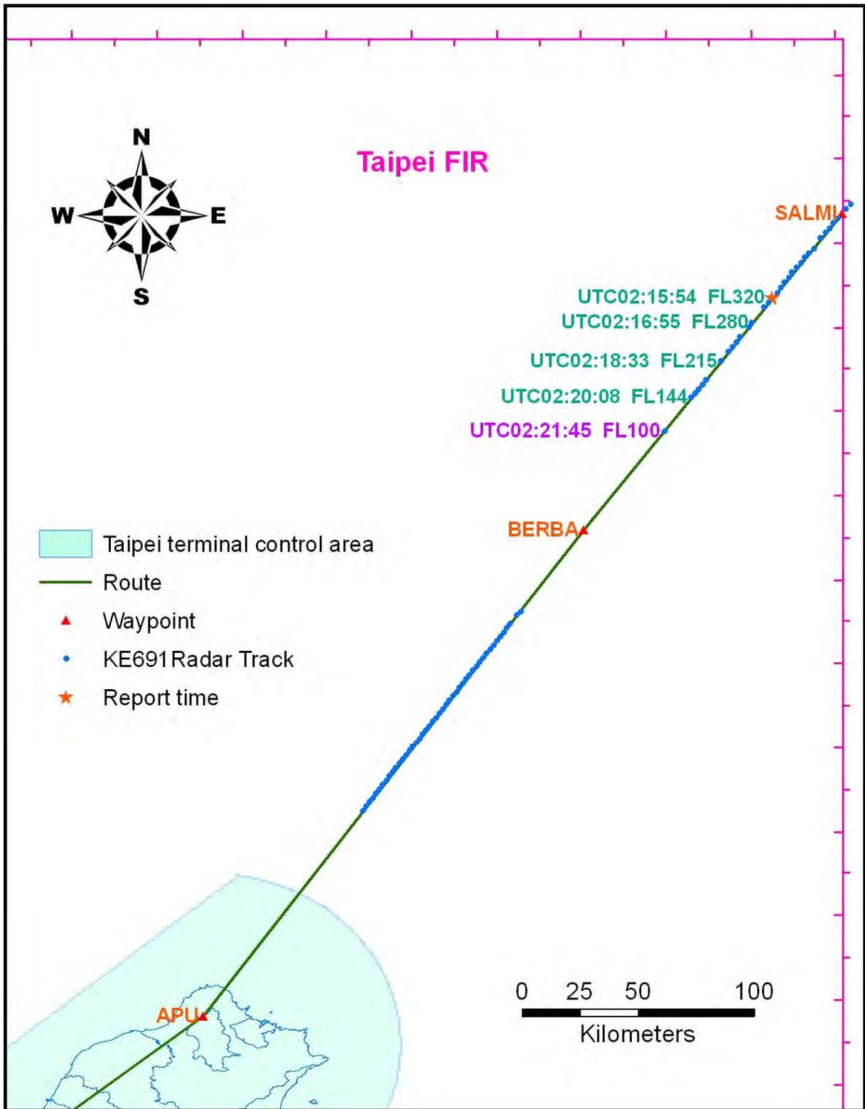
Fig. 4 Superposition of KE691 radar track and Taipei FIR chart
