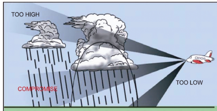
Figure 4-61 Tilt Setting Compromise
