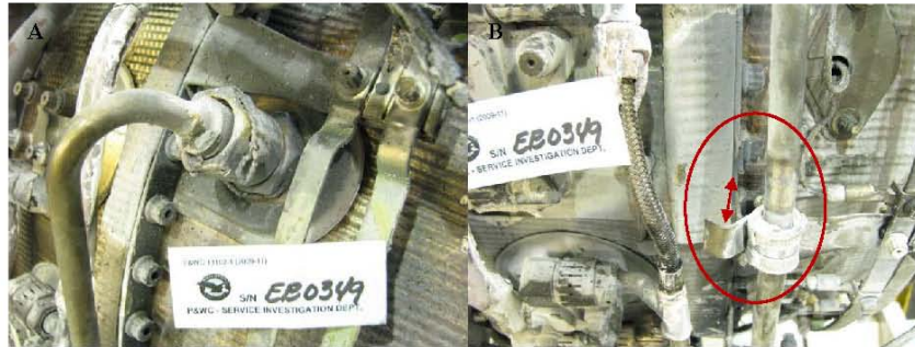
Photo no's 9 A & B Views of the tight-secured "B" nut (9 A) and fractured bracket (9 B) of the pressure tube assembly.
