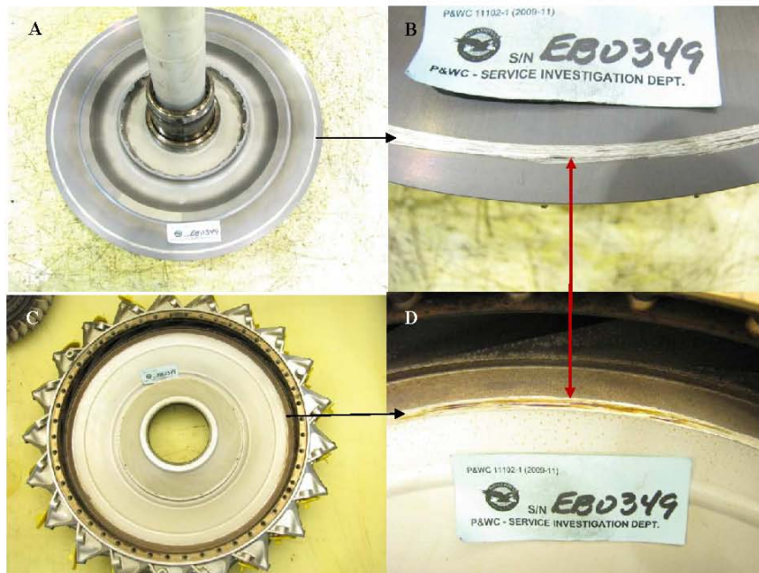
Photo no's 28 A to D Views of the rubbing of the LP impeller backface and diffuser case front wall.
