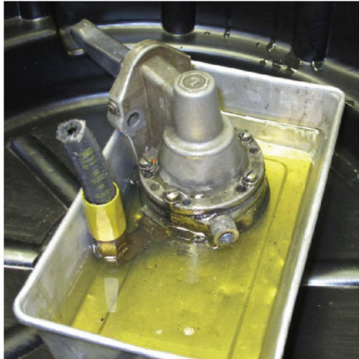
Figure 8- Fuel Pump Functional Check
