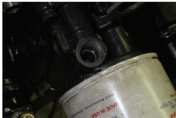
Figure 13- Breather Fitting, Fractured
