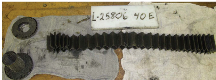
Figure 6- Oil Filter, Sectioned- Good Condition
