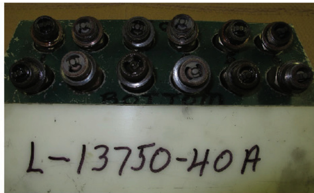
Figure 59- Engine Spark Plugs- Good Condition
