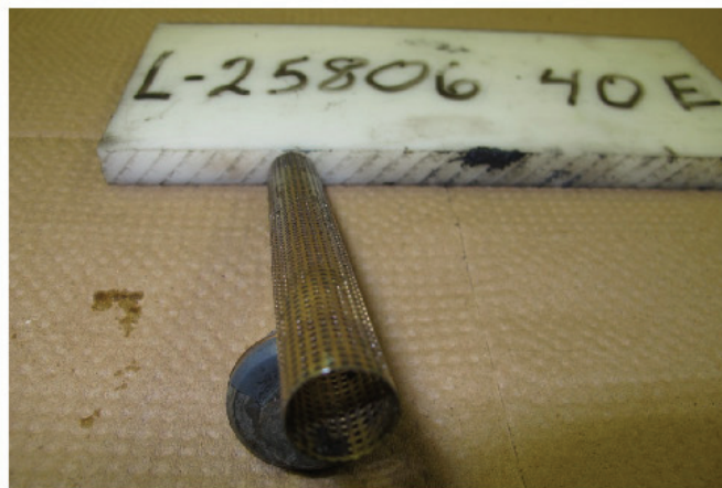
Figure 5- Oil Suction Screen- Clear
