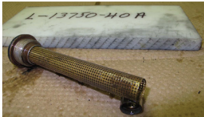
Figure 17- Oil Suction Screen- Clear
