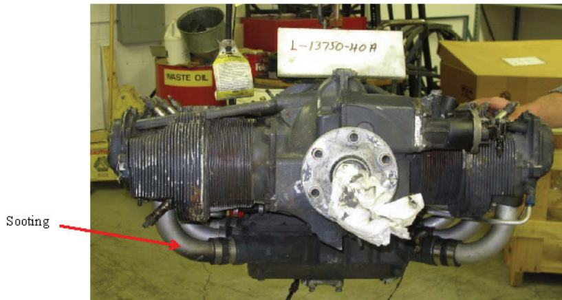
Figure 12- Localized Sooting on the No. 1 Cylinder Intake Pipe
