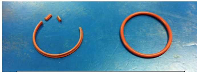
Left: Broken and brittle O-ring found on the SN 00715 Right: New O-ring (supply by OEM)
