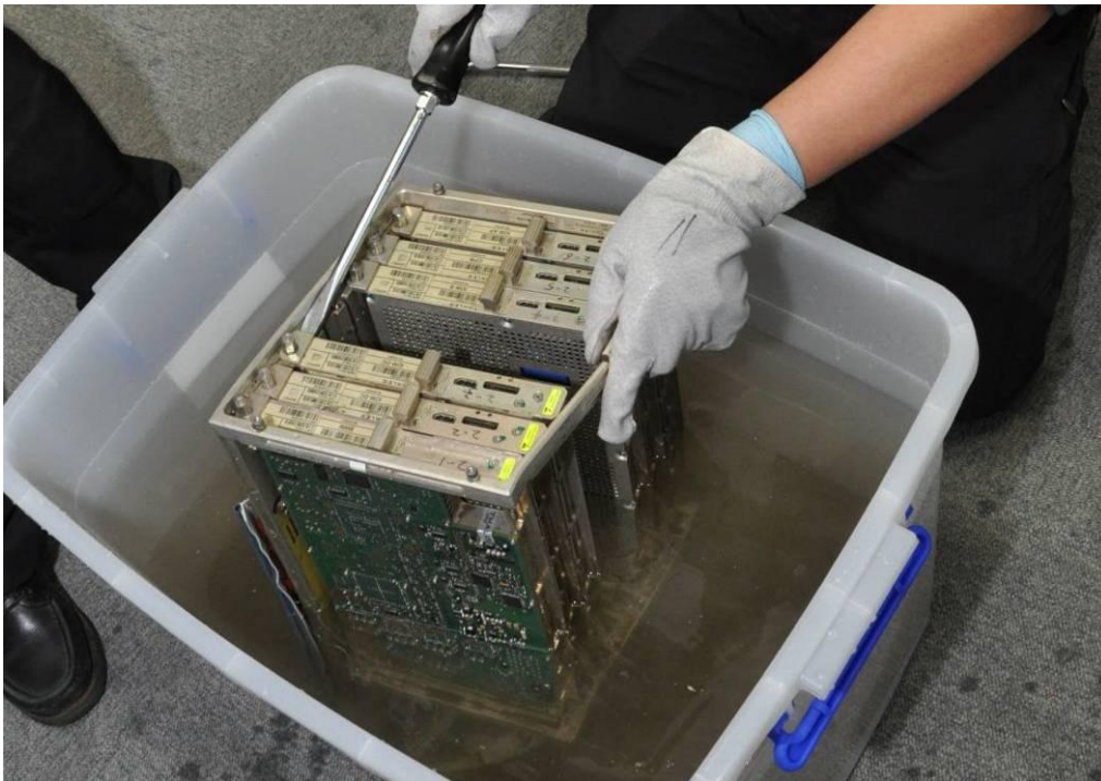
Figure 1.16-1 PCBs teardown from CAC rack
