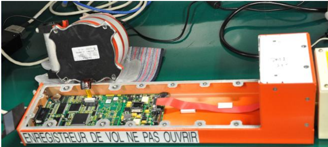
Figure1.11-5 Connecting the CSMU of GE235 FDR to chassis
