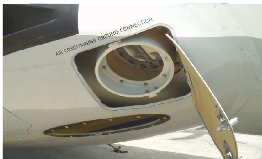
Figure 1.6-3 Exterior of the Ground Connection Check Valve
