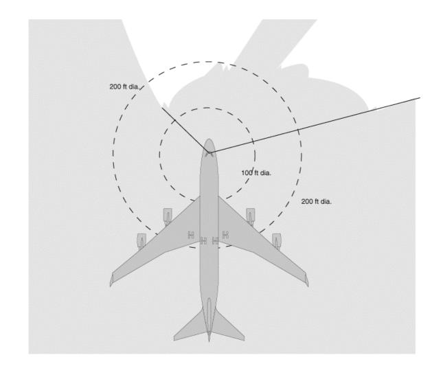
Figure 1.16-9 The ground visibility for Captain's eye reference points – wiper area only. The gray area represents the area not visible from Captain's eye reference points. The concentric circles do not represent the perceptual range of the human eye.
