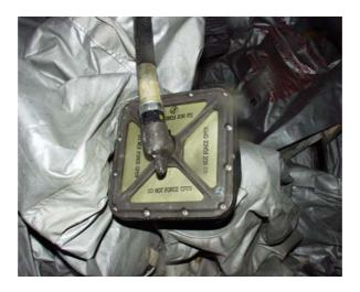
Figure 1.12-10 The aspirator of Door 2L slide
