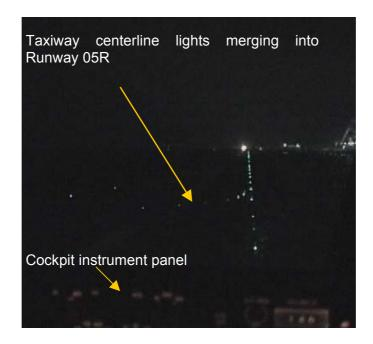
Figure 1.16-2 Taxiway centerline lights merged onto Runway 05R from Taxiway N2 (field of view from Boeing 747-400 cockpit-captain side)
