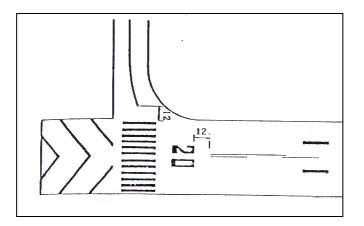
Figure 1.10-7 Taxiway centerline marking diagram
