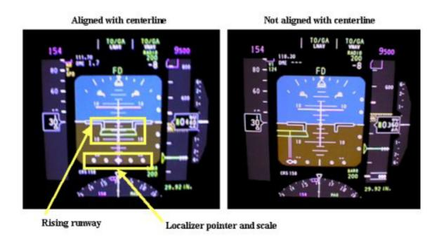
Figure 1.18-3 PFD indications associated with tuning the ILS.
