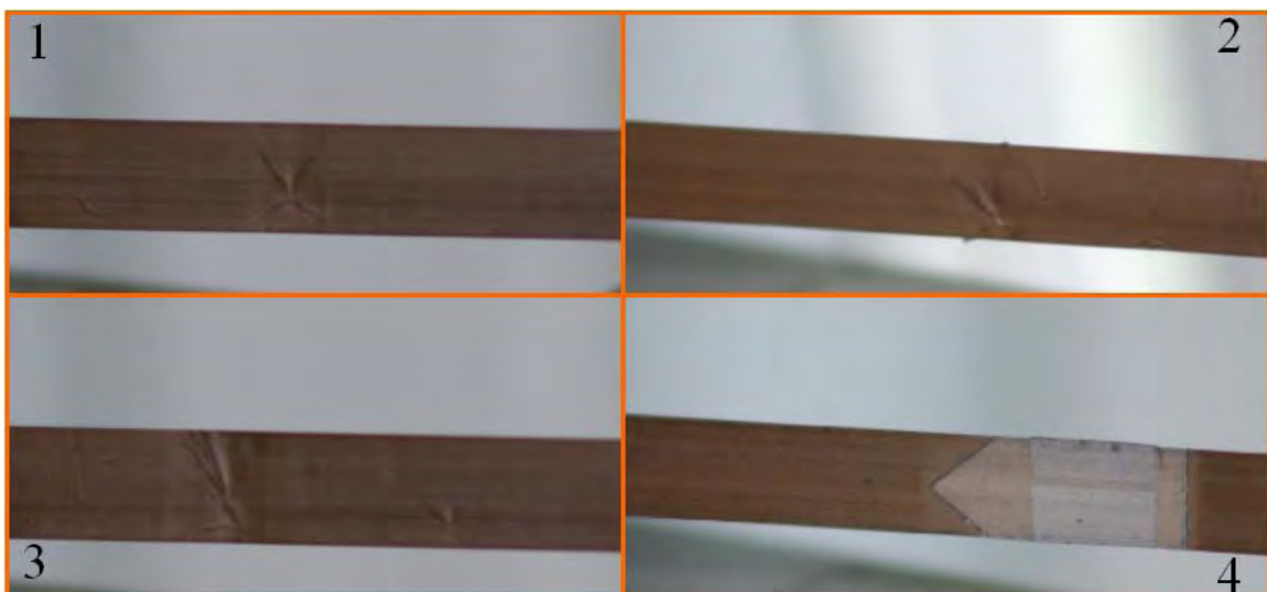
Figure 2.6-1 Damaged and spliced tape areas
