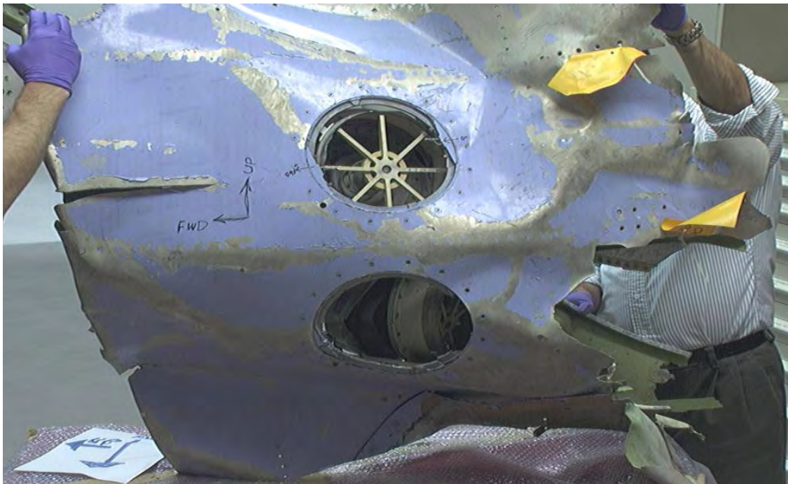
Figure 2.7-3 Pressure relief valves.
