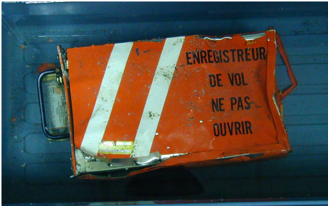
Figure 1.11-1 Damaged CVR in the water cooler
