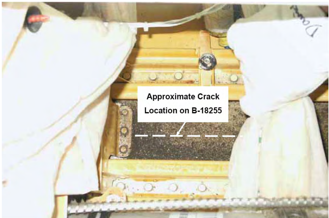
Figure 1.6-13 A B747-400 aircraft bilge area without removing CIC and dust
