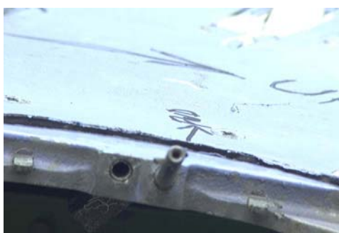
Figure 103: Forward/upper hinge pin, physically rotated by hand so that bent portion was oriented outboard.
