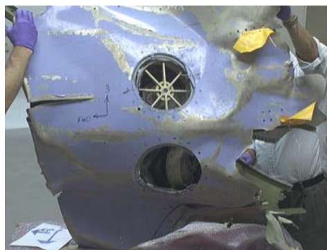
Figure 5 : Pressure Relief Valves
