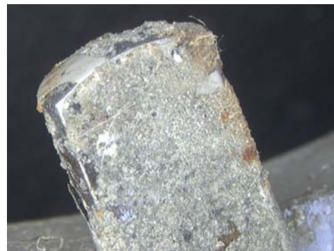
Figure 120 : Forward/upper stop pin, close-up of figure #119.
