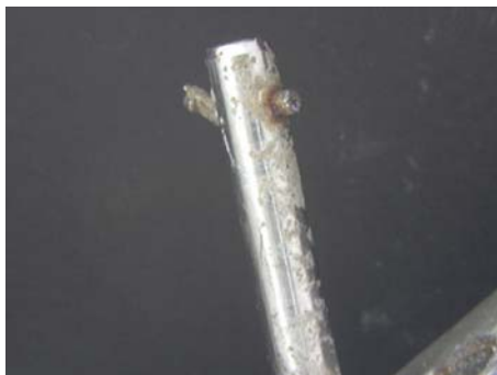
Figure 105: Detail of forward/upper hinge pin end.
