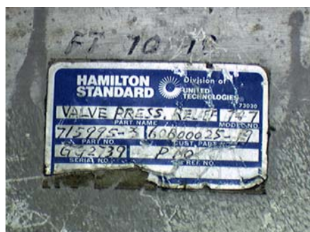
Figure 175: Lower Pressure Relief Valve, data plate identification.
