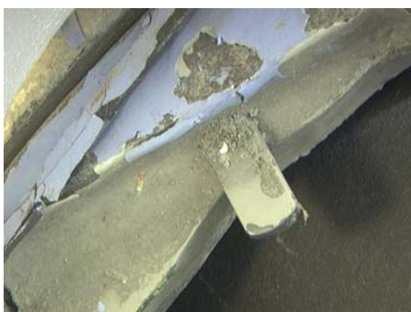
Figure 207: Forward/lower, stop pin as viewed form outside.
