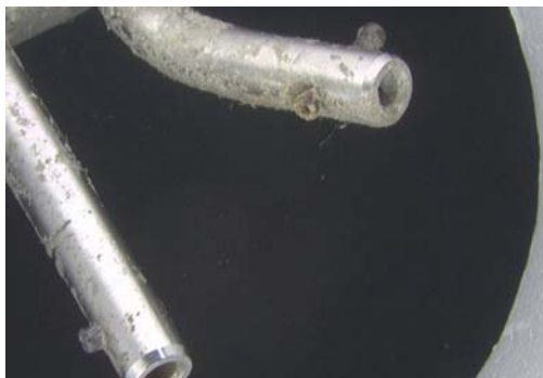
Figure 110: Aft hinge pins, upper & lower. Aft/lower pin is rotated to non-closed door position.
