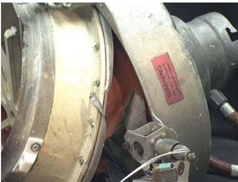
Figure 232 : Side view of gate assembly & valve cover, showing the approximate 30° angle between gate assembly & valve cover.
