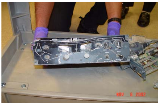
Figure 2 : Flight Engineer's Cabin Pressure Control Selector Panel
