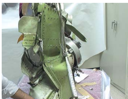
Figure 80: Frame, centerline (C/L) of stringer 31, looking fwd (frame view station 780).
