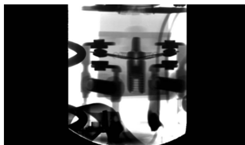
Figure 266: New switch, open valve, closed contacts.
