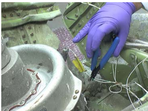
Figure 88: Prior to cutting switch lead wires.
