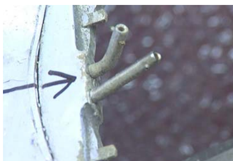
Figure 107: Aft hinge & stop pins, (looking from outside to inside) • Aft/upper hinge pin (lower pin in photo) is difficult to rotate. • Aft/lower hinge pin (upper pin in photo) rotates.
