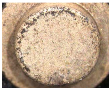
Figure 58: Stationary contact of oxygen control switch ("RESET" position).
