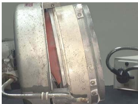
Figure 149: Offset angle between valve housing and gate.
