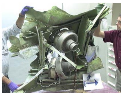
Figure 79: Upper & Lower Pressure Relief Valves, as installed, as viewed from inside.
