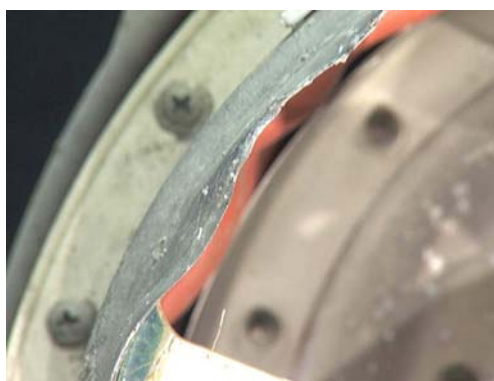
Figure 139: Close-up of knife-edge damage.
