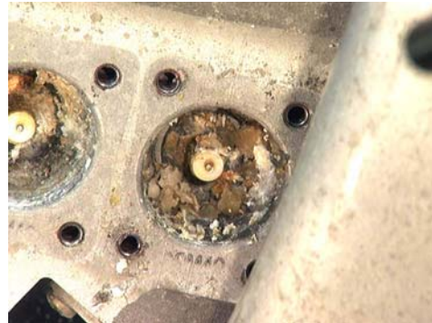
Figure 254: Integral sensor housing bore. • Heavy deposits. • Poppet appears to be frozen. • Salt deposits on end of poppet.
