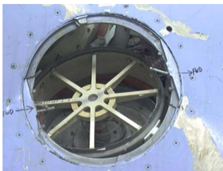
Figure 82: Upper Pressure Relief Valve, close-up showing markings.
