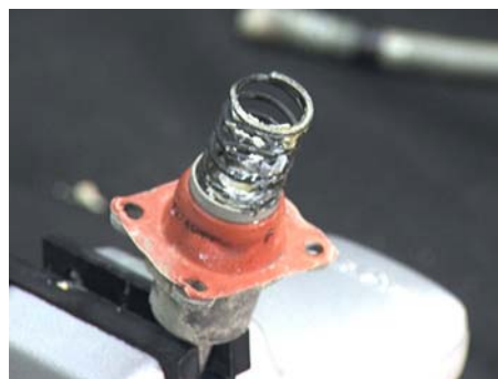
Figure 166 : Diaphragm appears to be intact.
