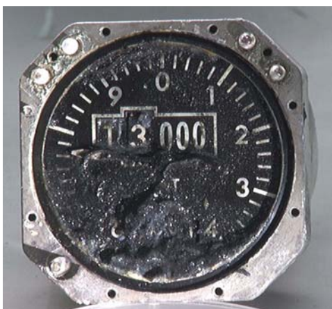
Figure 43: Cabin Altimeter Indicator, glass bezel removed
