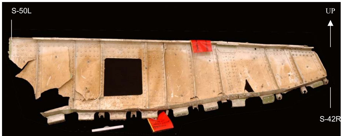
Figure 84. As received condition of the STA 2040 frame segment submitted for examination. The aft surface is shown.
