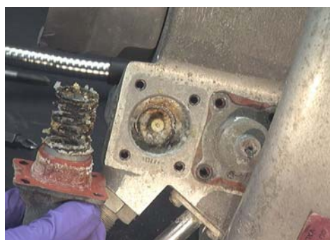
Figure 250: Showing remote ambient sensor removed.
