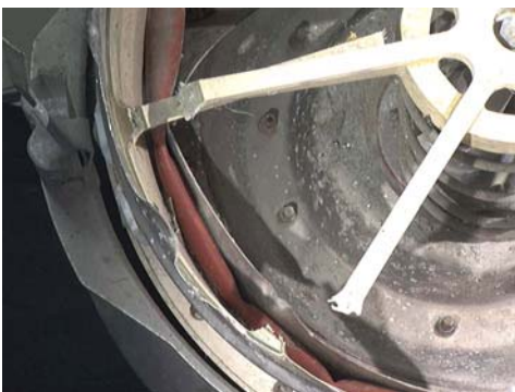
Figure 234 : Outer diaphragm, intact (not torn) portion.
