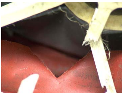
Figure 229: Outer diaphragm, torn location.
