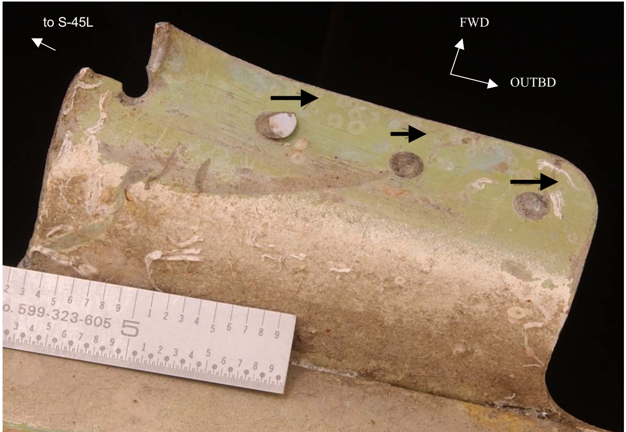
Figure 94. Shear tie between S-45L and S-44L of STA 1940 frame segment. Black arrows indicate the direction of loading.
