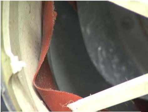
Figure 230 : Outer diaphragm damage.
