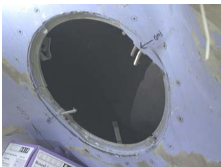
Figure 92: Upper Pressure Relief Valve, pins in approximately "door closed" position.
