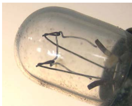
Figure 41: PRESS RELIEF light, lower right lamp. • Filament appears to be intact. • Legend plate missing, (Ref. Figure 37, red arrow for lamp location).
