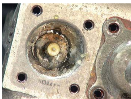
Figure 251: Close-up of salt deposits inside housing bore.
