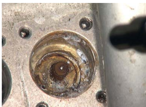
Figure 170: Integral ambient sensor poppet housing bore. • Poppet was free.
