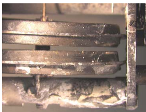
Figure 47: Cabin Altimeter Indicator, bellows displacement
