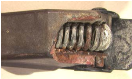
Figure 61: Top view of switch guard damage.
