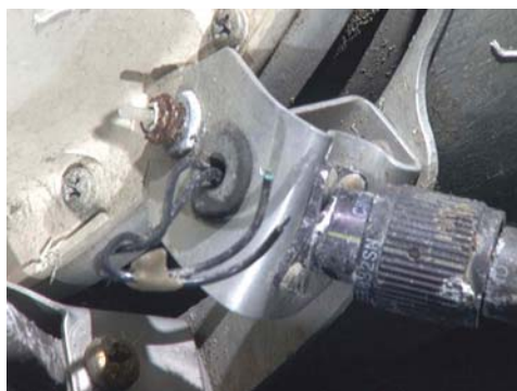
Figure 151: Switch mounting bracket, gate is against bracket.
