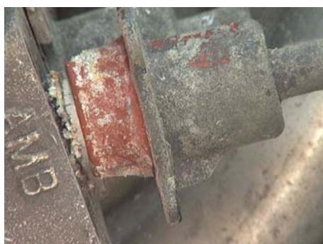
Figure 249: Remote ambient sensor, cover and diaphragm partially removed.
