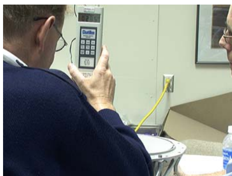
Figure 267: Comparison unit*, door A tension, 2.85 pounds (opening force from center edge of door).
