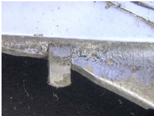
Figure 136: Aft/lower stop pin. • Overall, pin is relatively straight.
