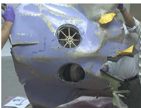
Figure 78: Upper & Lower Pressure Relief Valves, orientated as installed on airplane, [vertical centerline (C/L) through both valves at station 770].
