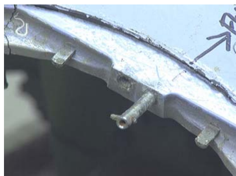
Figure 102: Forward stops and hinge pins, (looking from outside to inside). • Forward/upper hinge pin can rotate freely. • Stop pins look normal and unbent.
