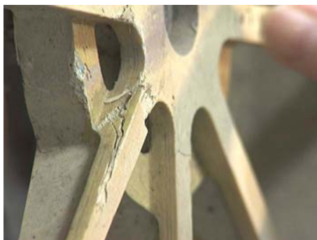
Figure 144: Worst of the center web cracks. 2 of 8 appear to be intact, remaining exhibit various degrees of cracking.
