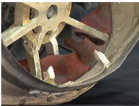
Figure 220 : Detail of more broken webs.
