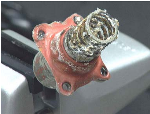
Figure 255: Integral sensor spring and diaphragm. • Heavy salt deposits. • Diaphragm intact. • Spring has heavy salt deposits and possibly salt corrosion.
