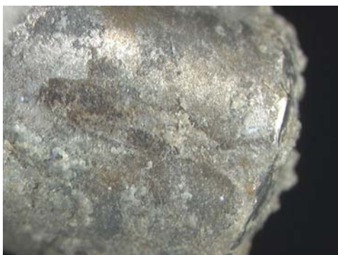
Figure 124 : Aft/upper stop pin, close up of figures #122 & #123, after pin was cleaned with alcohol.
