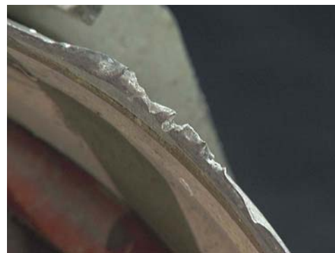
Figure 221 : Knife-edge close-up of damage.
