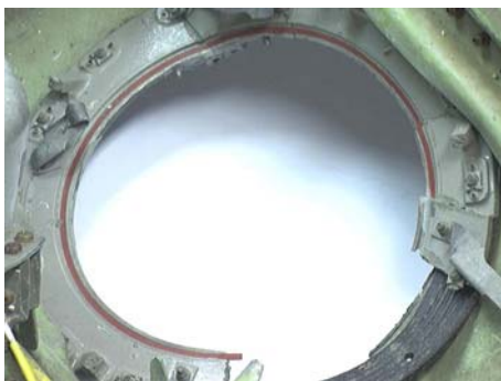
Figure 193: Non-metallic washer (gate seal), HS P/N 527355-13, as viewed from inside.
