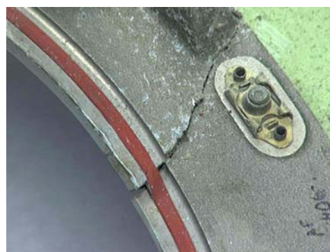
Figure 98: One slight cut adjacent to housing fracture.
