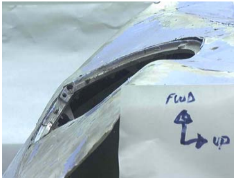
Figure 183: Skin distortion at valve mounting location.
