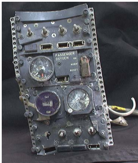
Figure 51: Flight Engineers Panel, overview. Includes modules M179, M183, M184 & M557.
