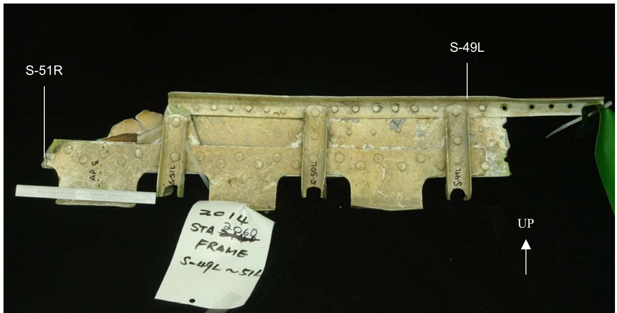
Figure 81. As received condition of the STA 2060 frame segment. The forward surface is shown in this view.
