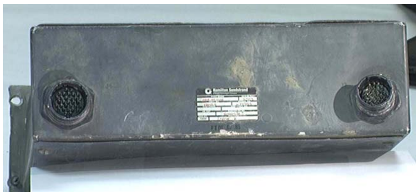
Figure 8: Flight Engineer's Cabin Pressure Control Selector Panel - (back view)
