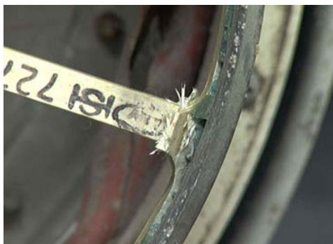
Figure 142: Overview, close-up of typical web fracture.
