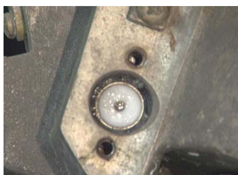
Figure 252: Remote ambient sensor, opposite end of poppet and guide.
