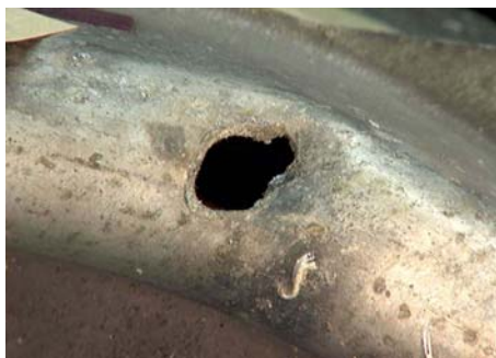
Figure 209: Hole penetrating support housing, HS P/N 727405-1.
