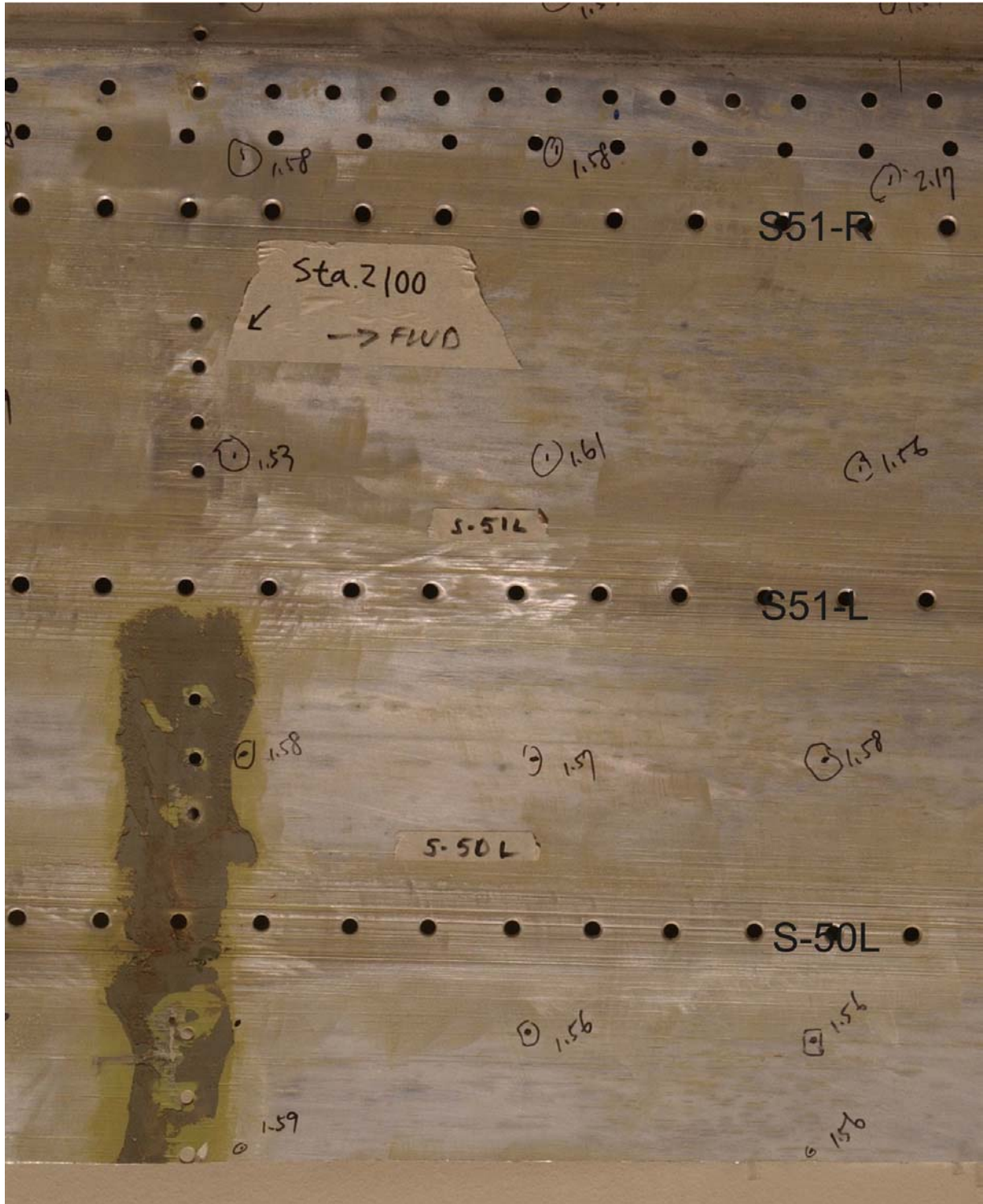
FIGURE 34. EXTENT OF DAMAGE CONSISTENT WITH A TAIL STRIKE
