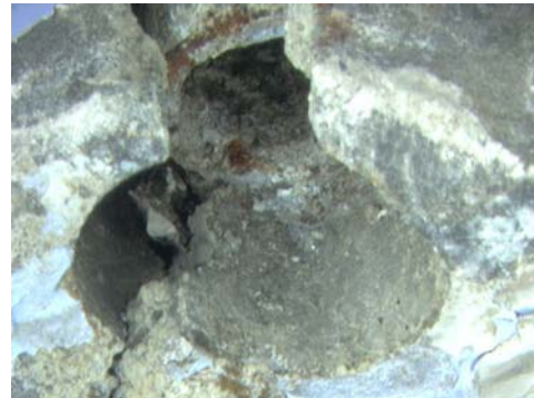
Figure 187: Forward/upper hinge pin, close-up of partial bushing.
