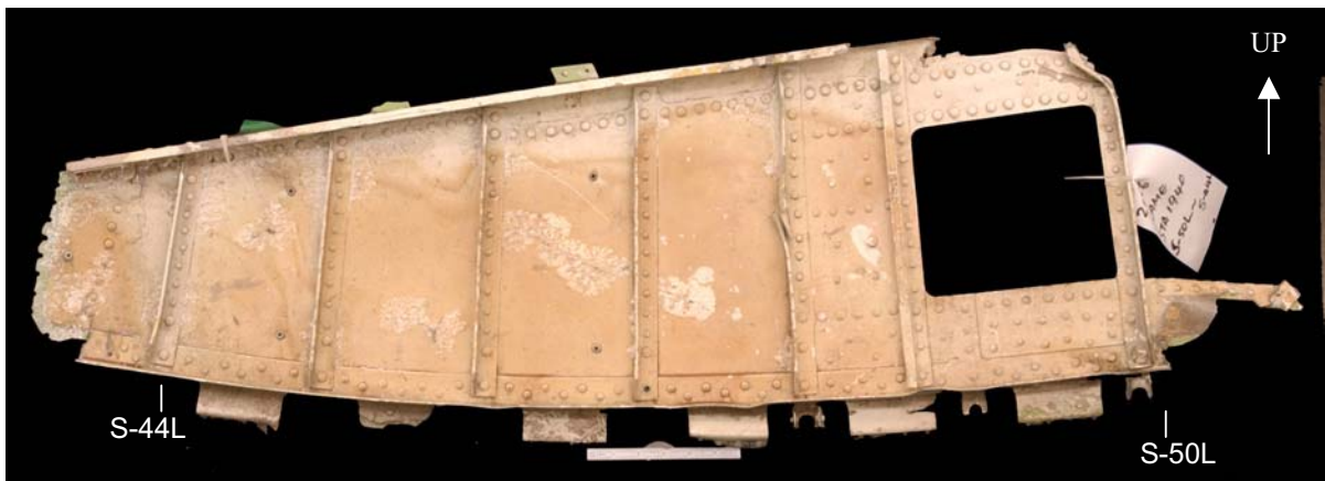
Figure 89. As received condition of the STA 1940 frame segment submitted for examination. The aft surface is shown in this view.
