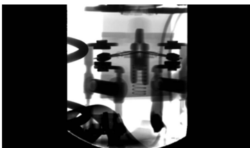
Figure 265: New switch, closed valve, not closed contacts.
