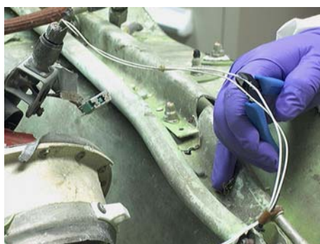
Figure 180: Lower Pressure Relief Valve. Cut switch lead wire A, step 1 in removal of lower valve (before cut).
