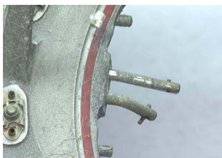
Figure 106: Aft hinge & stop pins (looking from inside to outside). • Aft/lower stop pin appears to have a rust mark and can rotate.
