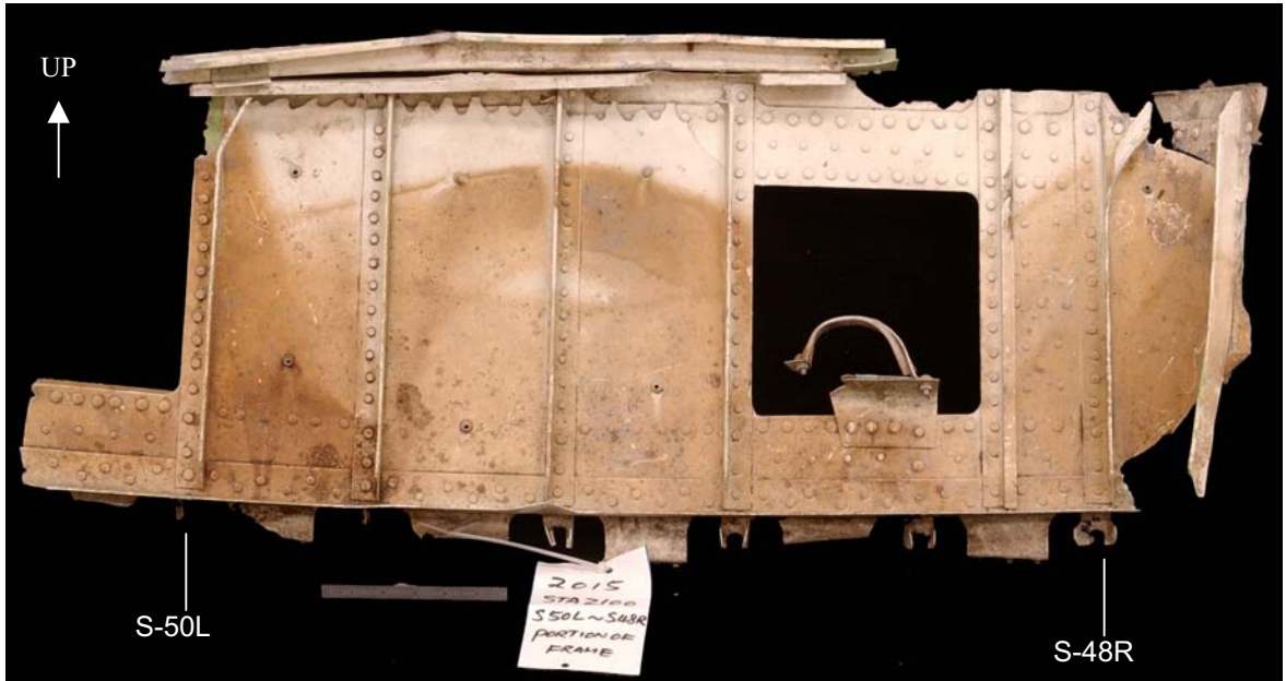
Figure 75. As received condition of the STA 2100 frame segment submitted for examination. The aft surface is shown in this view.
