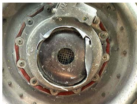
Figure 239: Overall of control, filter end.
