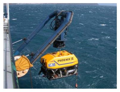
Figure 1.18-15 Salvage vessel- Ocean Hercules ROV
