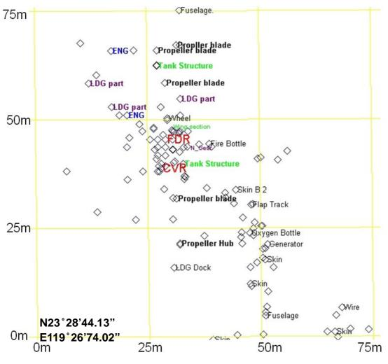
Figure 1.18-8 Wreckage distribution in dense area
