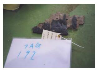
Figure 1.12-28 Wing de-icing boot
