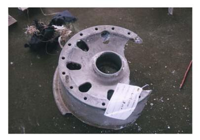
Figure 1.12-20 Broken wheel hub
