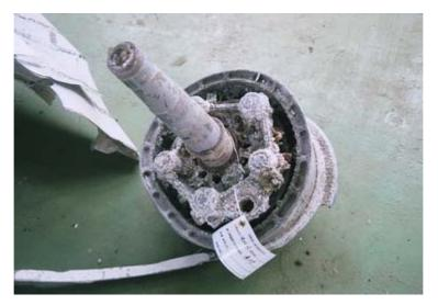
Figure 1.12-19 Wheel, axel and brake assy.
