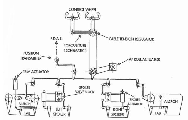
Figure 1.6-6 Roll control system diagram
