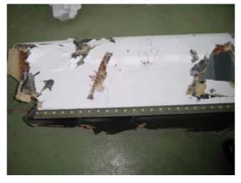
Figure 1.12-14 Rudder leading edge
