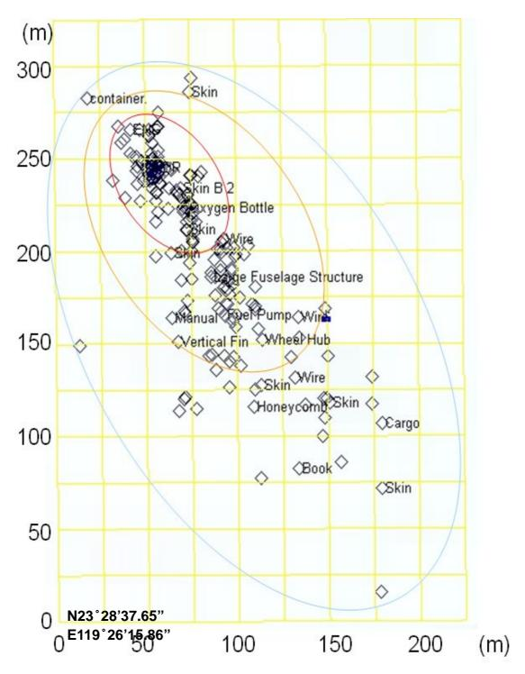
Figure 1.18-7 Wreckage distribution pattern
