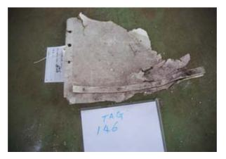
Figure 1.12-5 Cargo compartment partition
