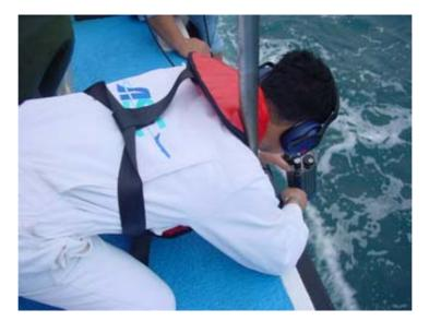
Figure 1.18-17 Search flight recorders with pinger receiver
