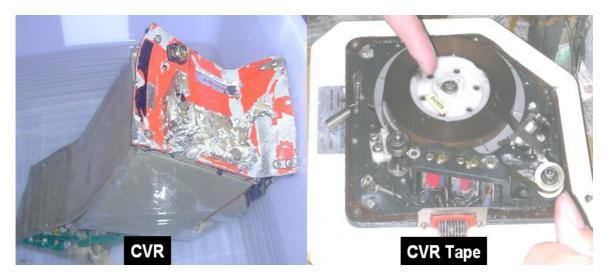
Figure 1.11-1 CVR physical damage and the CVR tape
