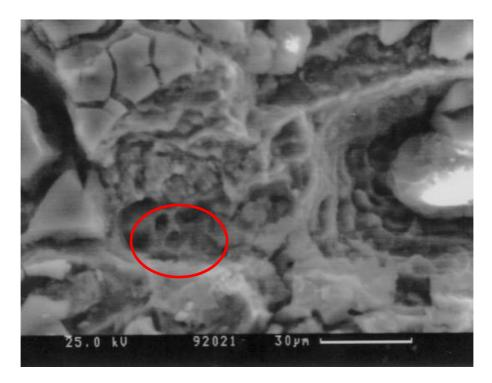
Figure 1.16-5 SEM examination showing the dimple structure (790X)  $_{\circ}$
