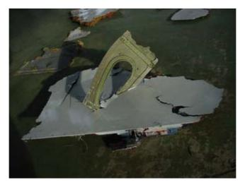
Figure 1.12-15 Window frame stuck into rudder
