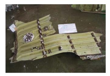
Figure 1.12-6 Wing root skin (bottom of fuel tank)
