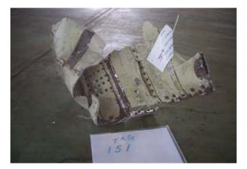
Figure 1.12-8 Wing trailing edge structure
