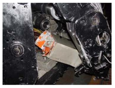
Figure 1.18-27 CVR recovered by ROV
