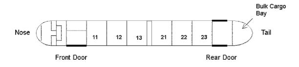
Figure 1.6-9 Schematics of ATR72 Cargo Bays
