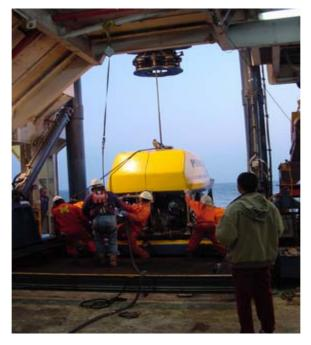
Figure 1.18-22 ROV operation on Ocean Hercules
