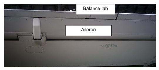
Figure 1.6-7 ATR72 aileron and balance tab
