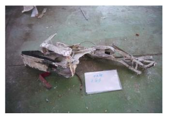
Figure 1.12-9 Flap driven mechanism
