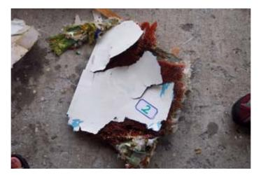
Figure 1.12-12 Vertical stabilizer honeycomb structure
