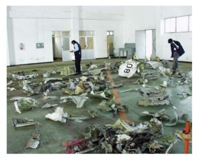
Figure 1.18-11 Underwater wreckage recovered by trawling operation
