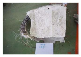
Figure 1.12-11 Flap leading edge structure
