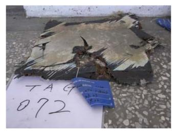
Figure 1.12-10 Flap honeycomb structure
