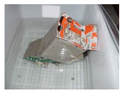
Figure 1.18-28 CVR closed view while recovered
