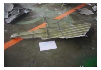
Figure 1.12-7 Wing tip structure (top of fuel tank)
