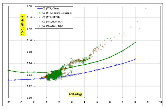
Figure 2.4-2 The extra drag of GE791 due to ice versus time (blue: clean configuration; green: de-icing boots inoperative; red: GE791 ice accretion)
