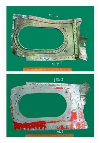
Figure 1.16-4 Wreckage with suspected fatigue crack
