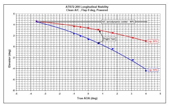
Figure 2.4-7 ATR 72-200 longitudinal stability
