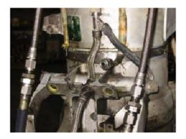
Figure 1.12-5LH MLG electrical and hydraulic systems damage
