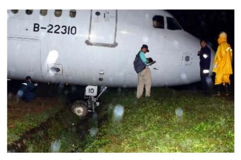
Figure 1.3-2 The NLG entered a drainage ditch (approx 1m deep)
