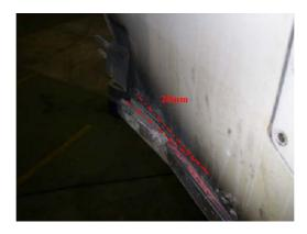
Figure 1.12-19 Twisting of the lower profile
