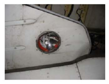
Figure 1.12-11 Landing light damaged
