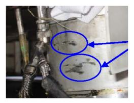
Figure 1.12-6LH MLG Scratches – max depth 0.5mm
