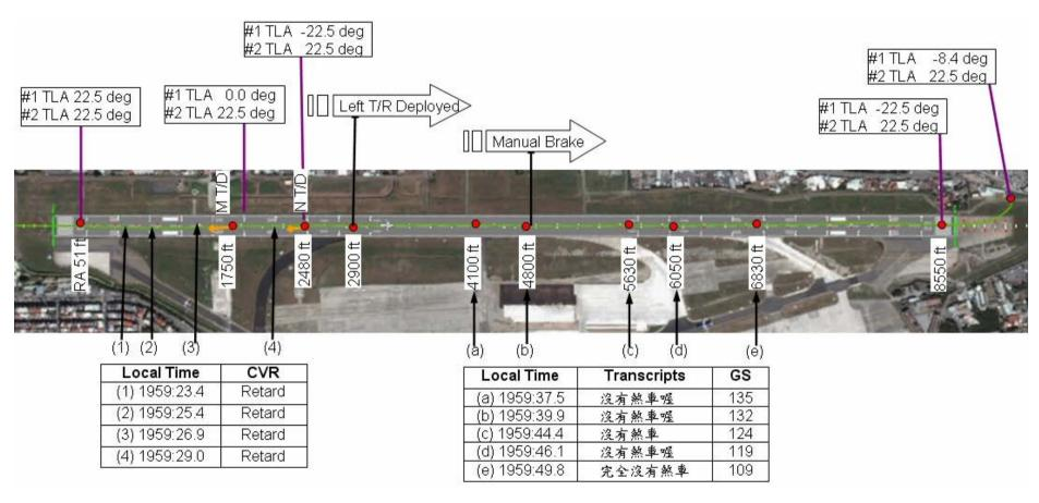
Figure 2.3-1 The relative locations determined by the CVR and FDR recorded data during landing phase.
