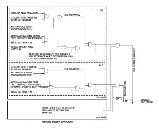
Figure 1.6-2 Ground spoiler activation logic diagram
