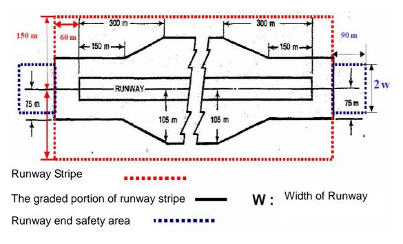
Figure 2.6-1 Runway Safety Area including aprecision approach runway when the code number is 3 or 4
