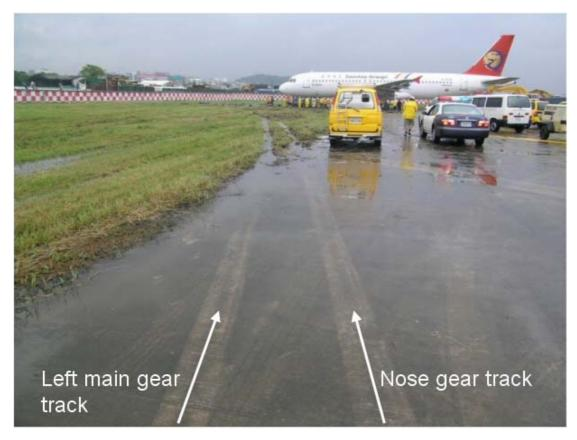
Figure 1.18-3Ground tracks from the stopway pavement to the grass area
