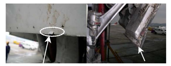
Figure 1.12-4Deformation and dent to NLG Aft doors
