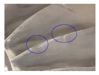
Figure 1.12-12 Fan damage
