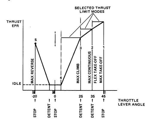
Figure 1.6-4Thrust control lever angle and associated function
