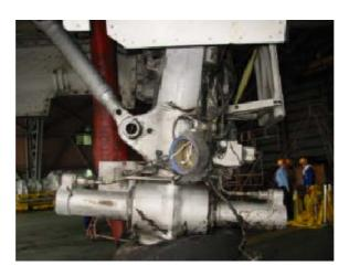
Figure 1.12-3NLG without broken sliding tube
