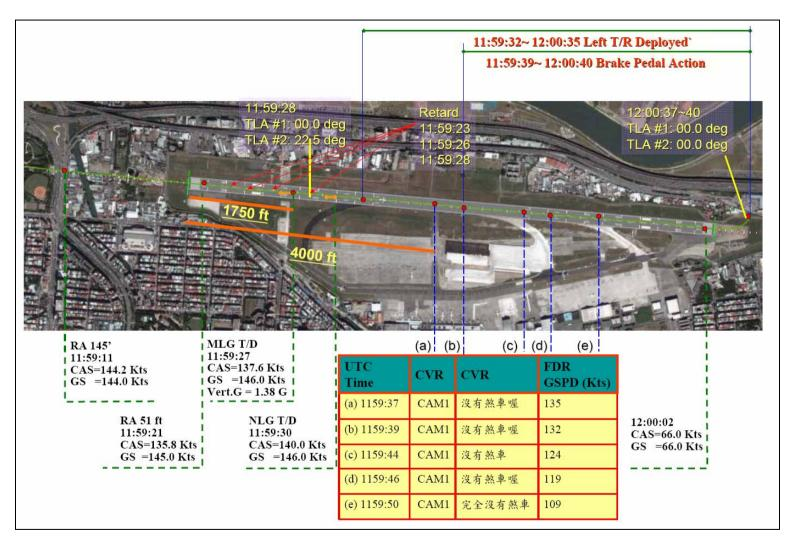
Figure 1.11-3 Superpose of Flight Path and Satellite Image (Time, Flight Path, FDR Parameters, and CVR Transcripts)
