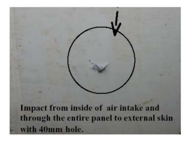
Figure 1.12-10 External Damage
