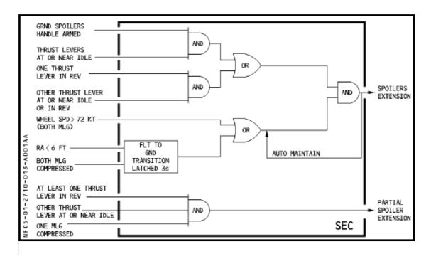
Figure 2.3-2 Ground Spoiler full extension logic
