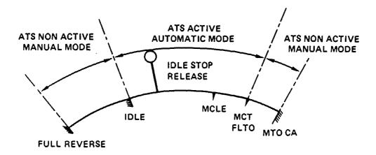
Figure 1.6-5Throttle control lever vs. manual/autothrust active area
