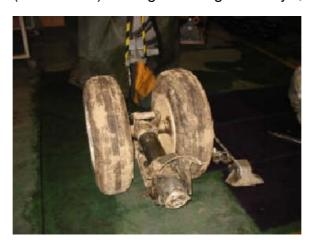
Figure 1.12-2NLG Sliding tube broken and associated harnesses destroyed
