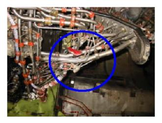
Figure 1.12-13 Bent Pipes, lower drain missing
