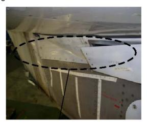
Figure 1.12-21 Fairings deformed
