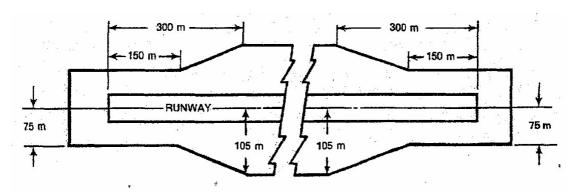
Figure 1.10-2Graded portion of a strip including a precision approach runway where the code number is 3 or 4
