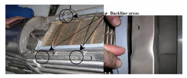
Figure 1.12-22 Upper cantilever angle buckling
