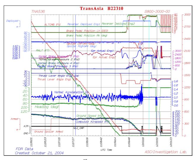
Figure 1.11-1 Flight Data Plot<sup>16</sup> (Final Approach, Landing and Deceleration)
