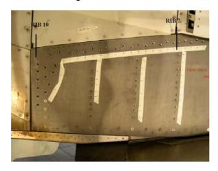
Figure 1.12-16 Lateral Panel Pulled fasteners
