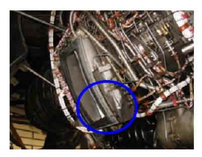
Figure 1.12-14 Lateral cooler damaged
