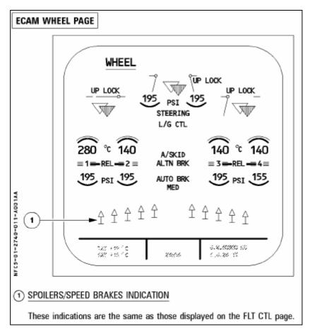
Figure 2.3-3An ECAM display shows the ground spoilers are extended
