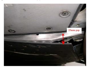
Figure 1.12-18 Internal profile deformed.
