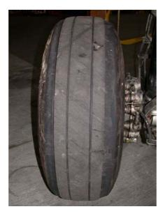
Figure 1.16-1 Deep cut damage and diagonal scratch marks
