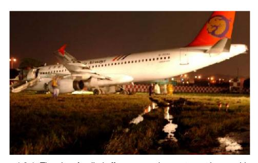
Figure 1.3-1 The aircraft rolled off runway and came to rest in a muddy area 90 degrees to the runway heading
