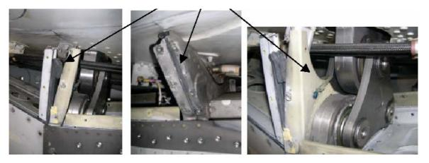
Figure 1.12-20 Vertical Profiles deformed
