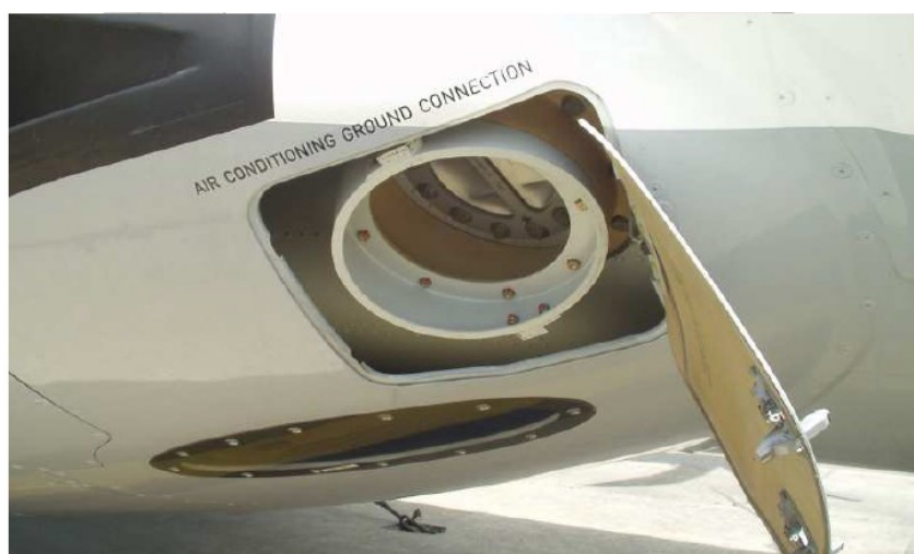
Figure 1.6-3 Exterior of the Ground Connection Check Valve
