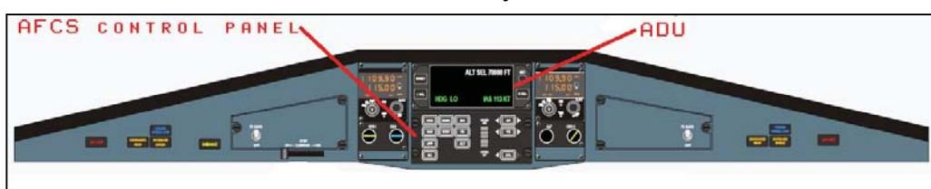
Figure 1.6-3 Automatic Flight Control System (AFCS)
