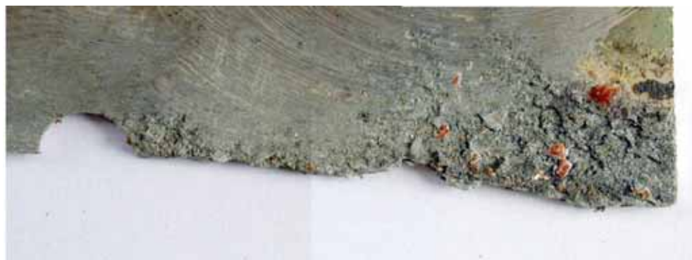
Figure 1.16-6 Exterior surface of the damaged skin
