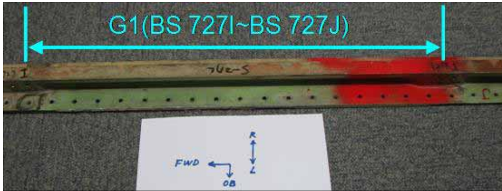
Figure 1.12-25 Stringer Corrosion Area G1
