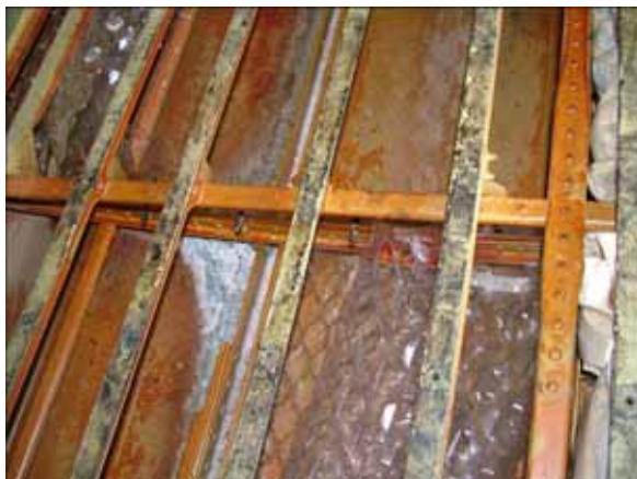
Figure 1.12-2 (F) Corrosion aft of Sta. 807
