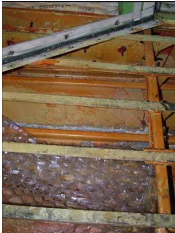
Figure 1.12-2 (N) Crack Rear End at Sta. 869.7 Cargo Compartment Interior View
