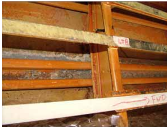
Figure 1.12-2 (M) Corrosion aft of Sta. 847
