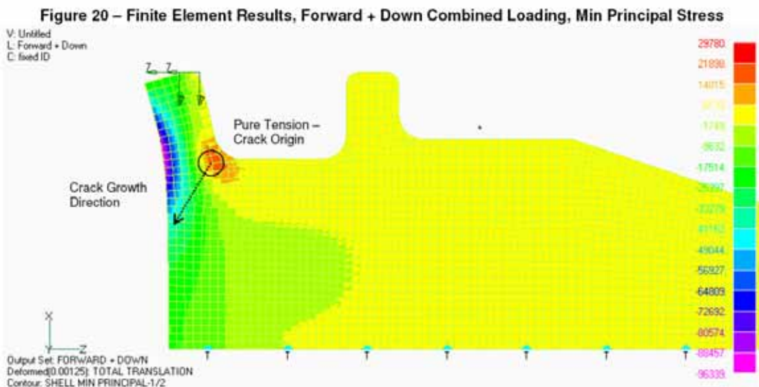
Figure 1.16-19 Mode 1 crack analyzed by FEA
