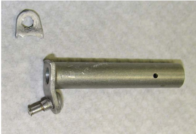
Fig. 1.12-26 The Broken Standoff
