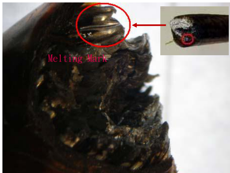
Fig. 1.14-4 Melting Mark of Metal Wire Due to Heat-2
