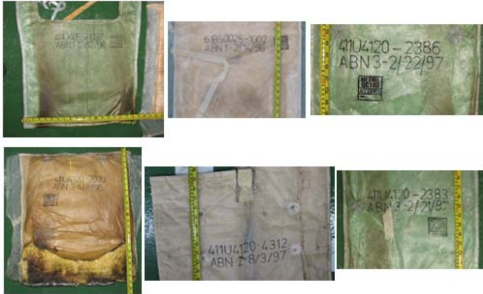
Fig. 1.14-5 Distinguishable Samples of Damaged Insulation Blankets
