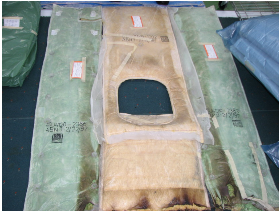
Fig. 1.12-4 Discoloration and Burnt Mark of the insulation Blanket
