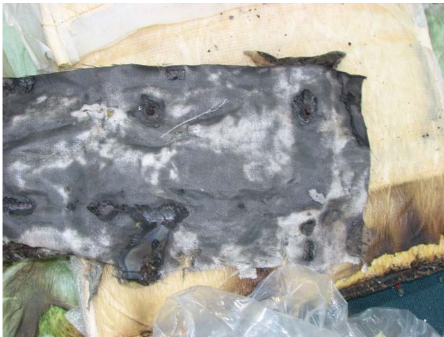
Fig. 1.12-5 Burnt and Carbonized Insulation Blanket
