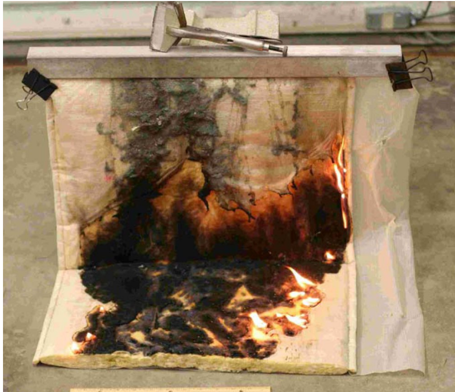
Fig. 1.16-7 Burn Test of Insulation Blanket
