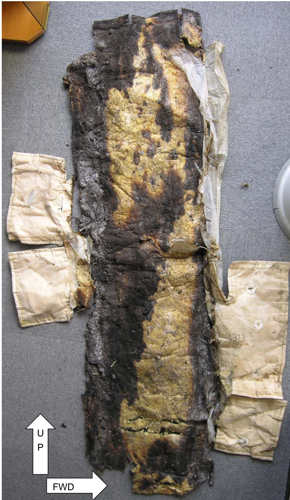
Fig. 1.12-7 STA 2020~STA 2040 Damaged Insulation Blanket IB Side
