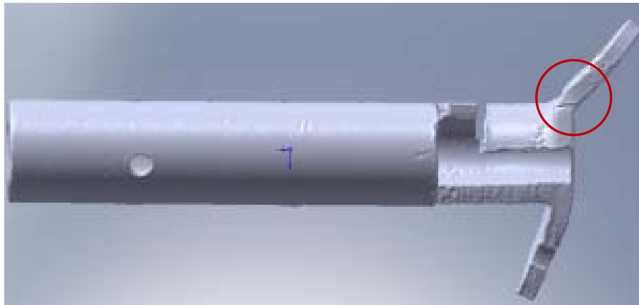
Fig. 2.1-3 a stereo lithography (STL) model of failure standoff
