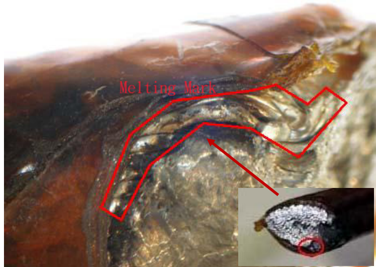
Fig. 1.14-3 Melting Mark of Metal Wire Due to Heat-1
