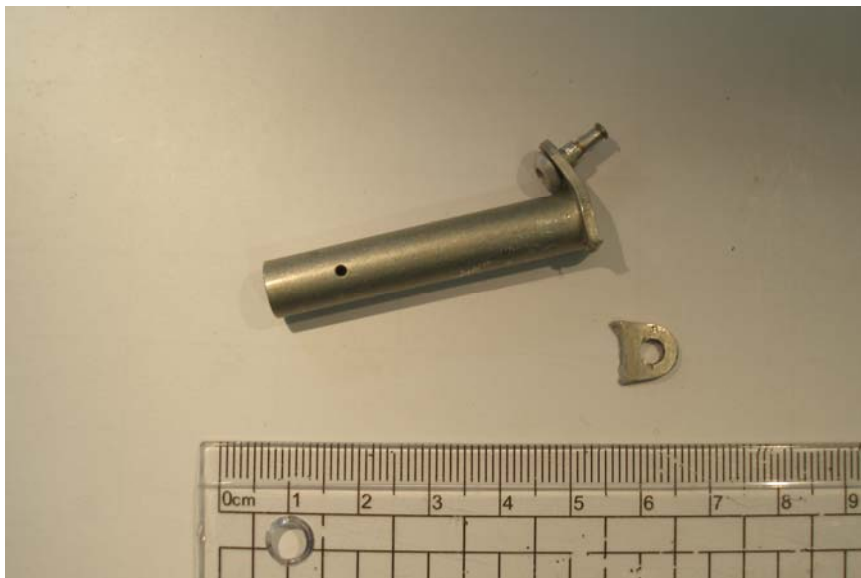
Fig. 1.16-1 the APU power cable standoff
