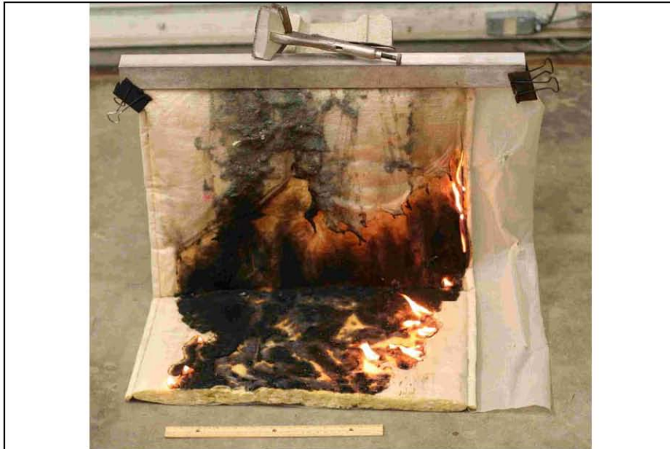
Figure 1. An initial alcohol-soaked cotton swab was dropped in the center of the flat area and the flame extinguished. When the flame went out, a small circular hole in the surface film existed in the center of the lower flat area shown. This photo shows a second test, in which a burning alcohol-soaked cotton swab was dropped near the left end of the fold. The visible creeping flame burned around and past where the initial flame stopped when this photo was taken.
