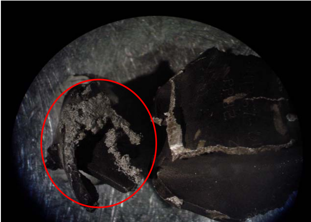
Figure 2.3-4 The precipitation and displacement of metal particles of impeller ( red line ) .
