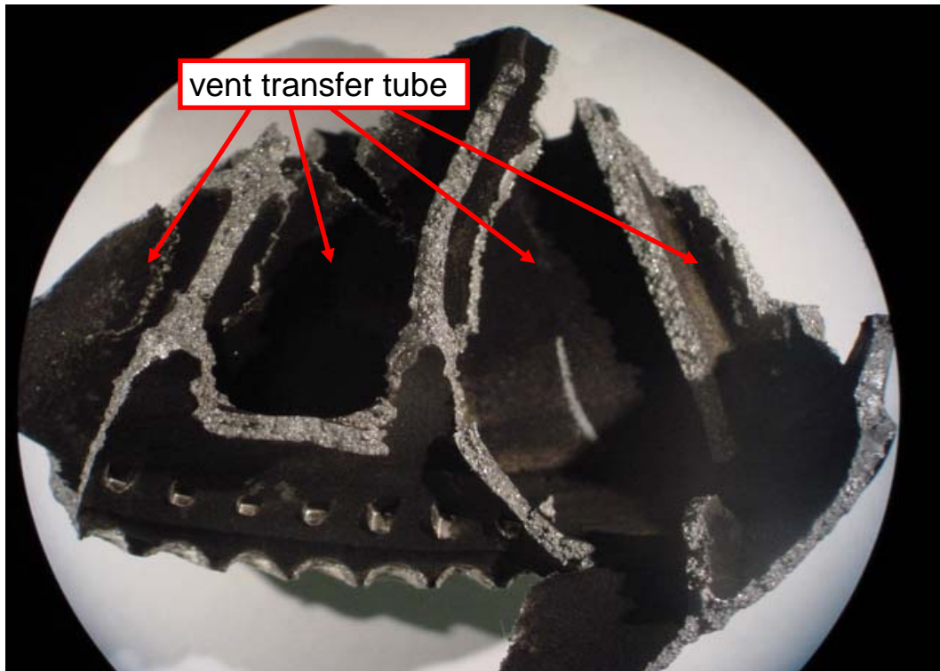
Figure 2.3-3 Black carbon deposits were found in the vent transfer tube inside the impeller
