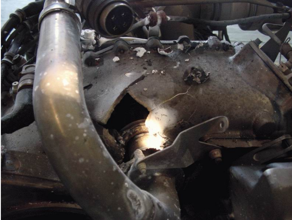
Figure 1.2-2 Perforation on the top right side of the rear inlet case
