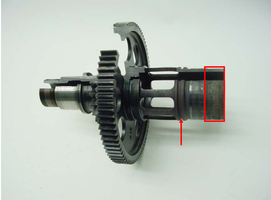
Figure 1.8-1 Location of the rubber seal (indicated by the red arrow) and the carbon seal (indicated by the red box).
