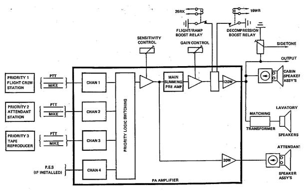
Figure 1.4-5 Priority Block Diagram
