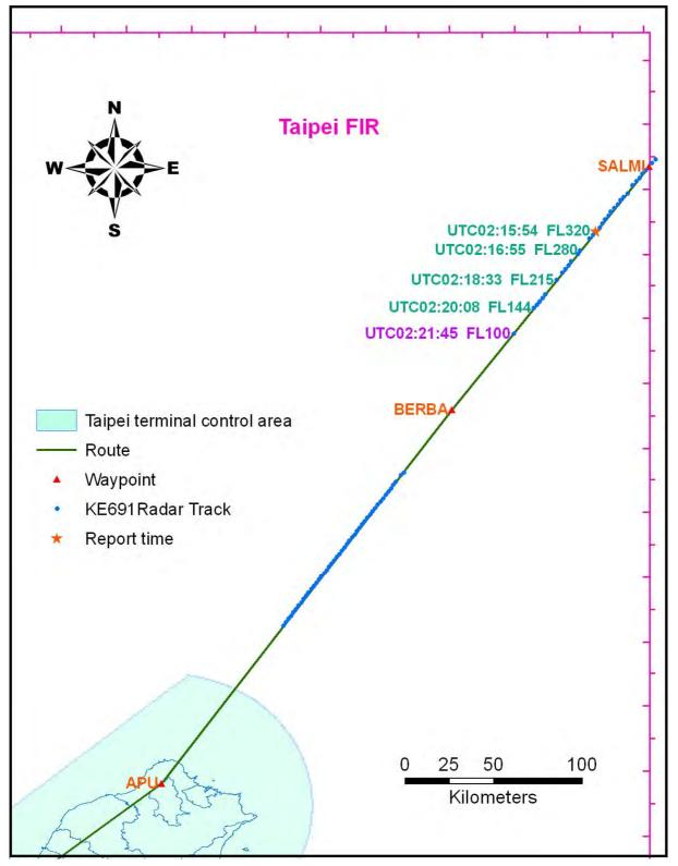
Fig. 4 Superposition of KE691 radar track and Taipei FIR chart (UTC 1055~1114, descent from FL320, approach, and Landing)
