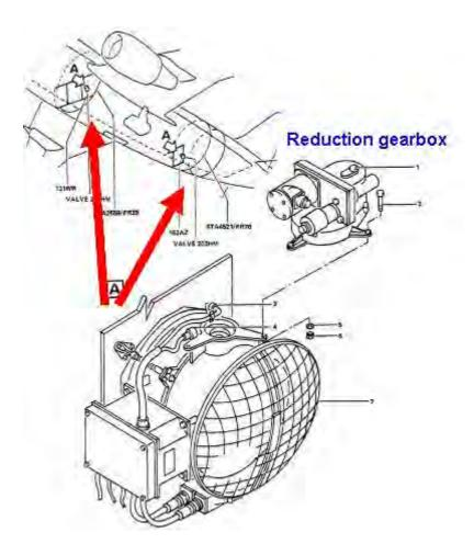
Figure 1.4-2 Pressure Control System
