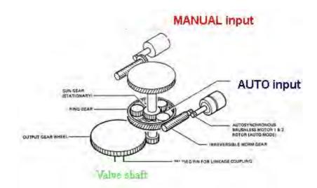
Figure 1.4-4 Out flow valve control modes
