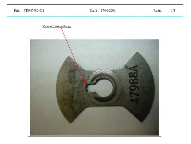
CONCLUSION: The broken flange explains the malfunction of the motor on both modes 1&2. It was randomly ordered by the variation of position of the flange. So, windings were not in accordance with sensors. This failure is considered as an isolated case.
