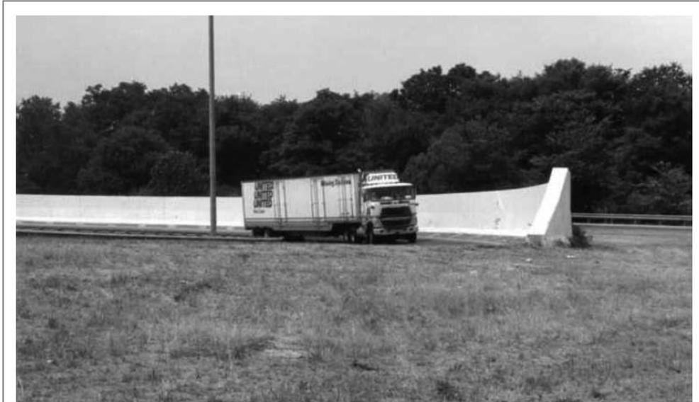
Figure 5-21. 2,290-mm [90-in.] New Jersey Barrier
