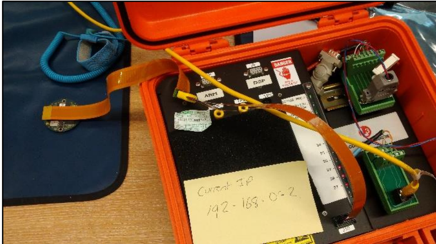
Figure1.10-4 S-VDR CSM memory download wiring condition
