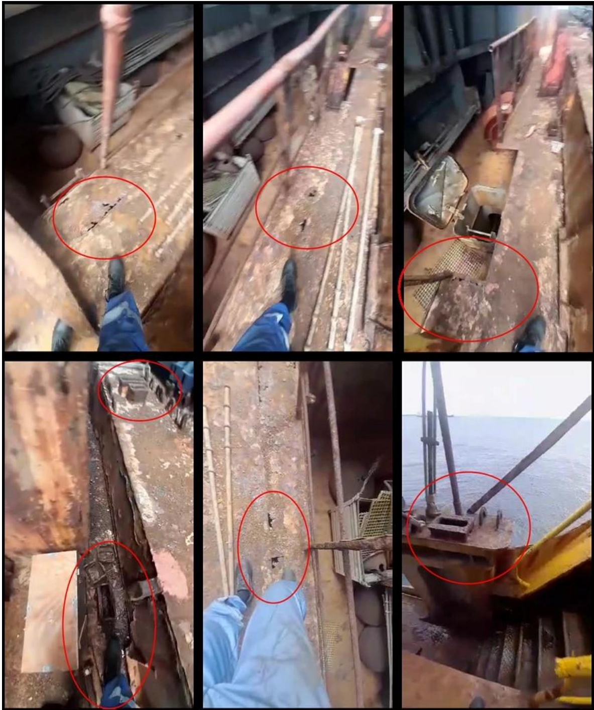
Figure1.11-2 Photos of holes and rust on ANGEL's main deck
