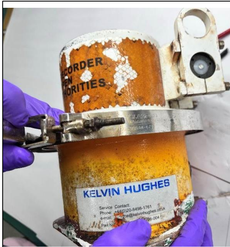
Figure1.10-2 Visual inspection of appearance of S-VDR CSM
