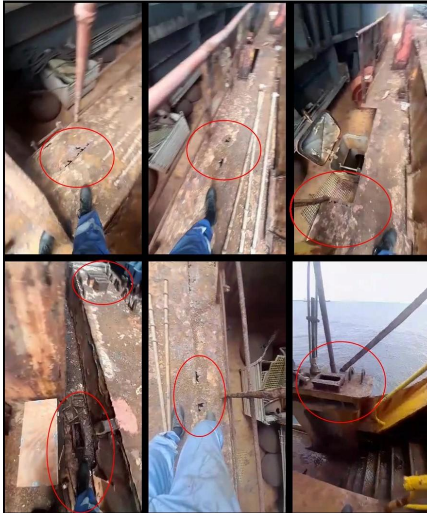
Figure1.11-4 Photos of holes and rust on the main deck of the ANGEL
