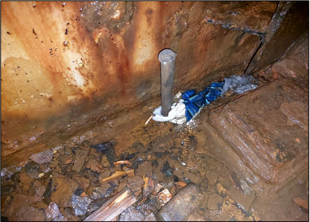
Figure 2.2-2 shows the ANGEL's crew using wooden plugs to temporarily seal the breaches in the cargo hold bottom sounding pipes.
