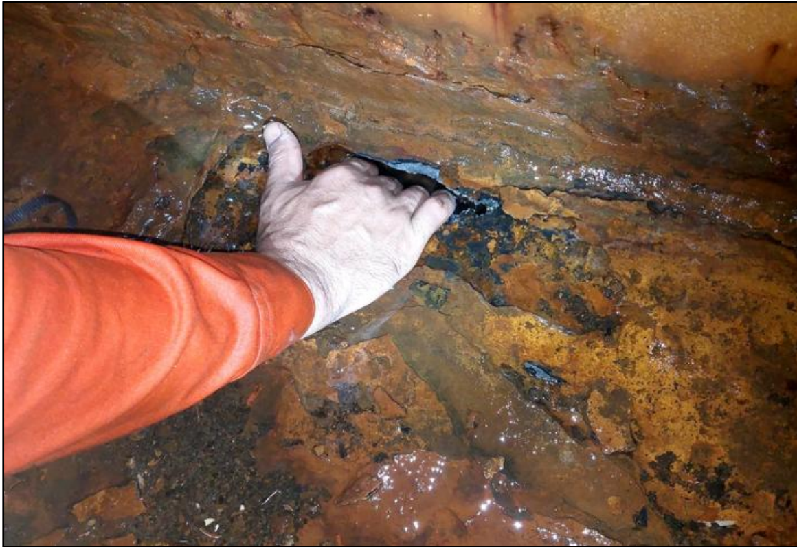
Figure 2.2-1 shows the appearance of the breached cargo hold bottom in the cargo hold no.3 of the ANGEL
