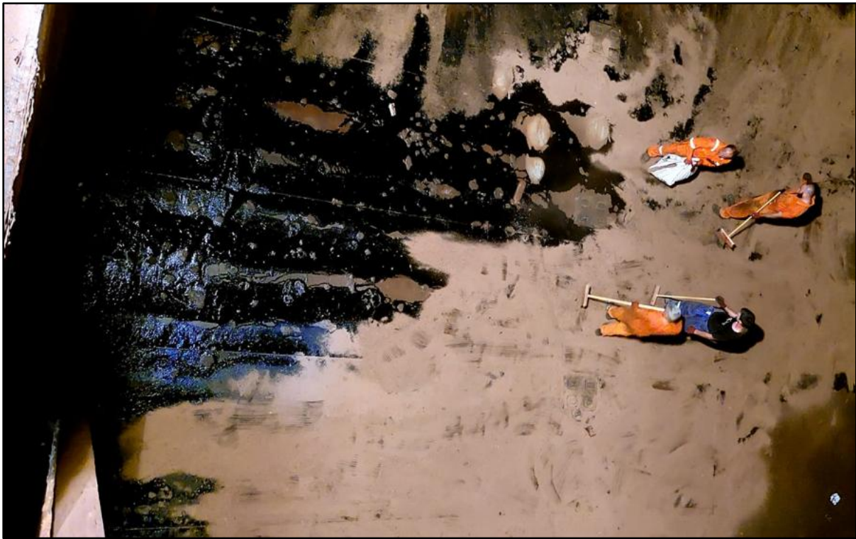
Figure 1.11-1 Crew cleaning up oil leakage in the cargo hold no.4
