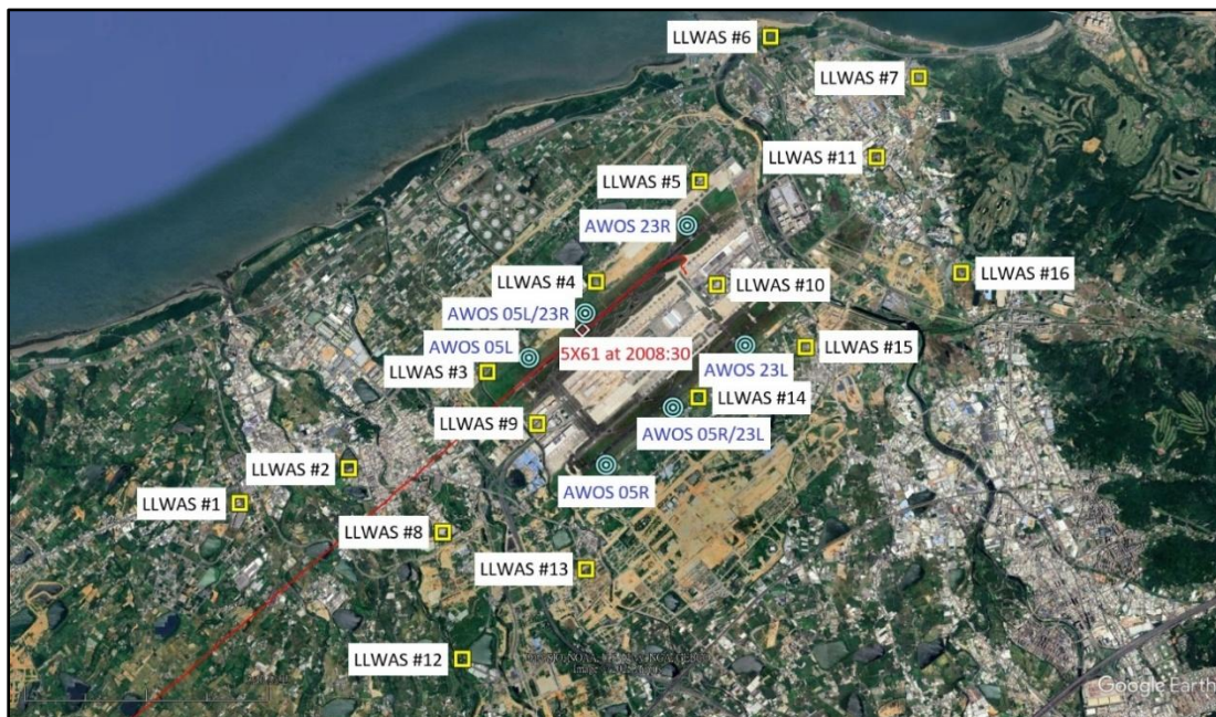
Figure 1.7-2 AWOS and LLWAS anemometer locations at RCTP
