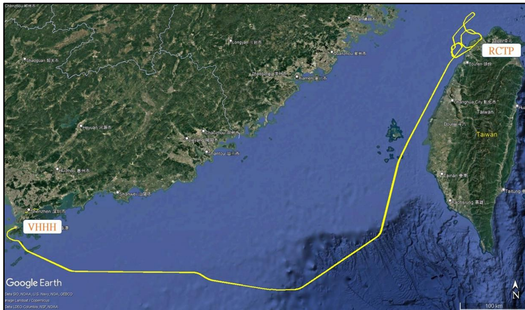
Figure 1.1-2 FDR recorded flight path of occurrence flight
