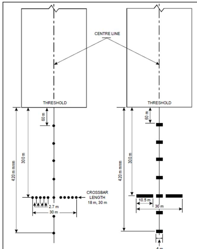
Figure 2.12-1 The typical simple approach lighting system
