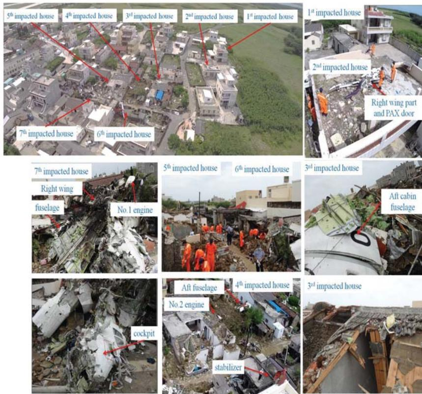
Figure 1.12-8 Aircraft main wreckage distribution and damaged buildings
