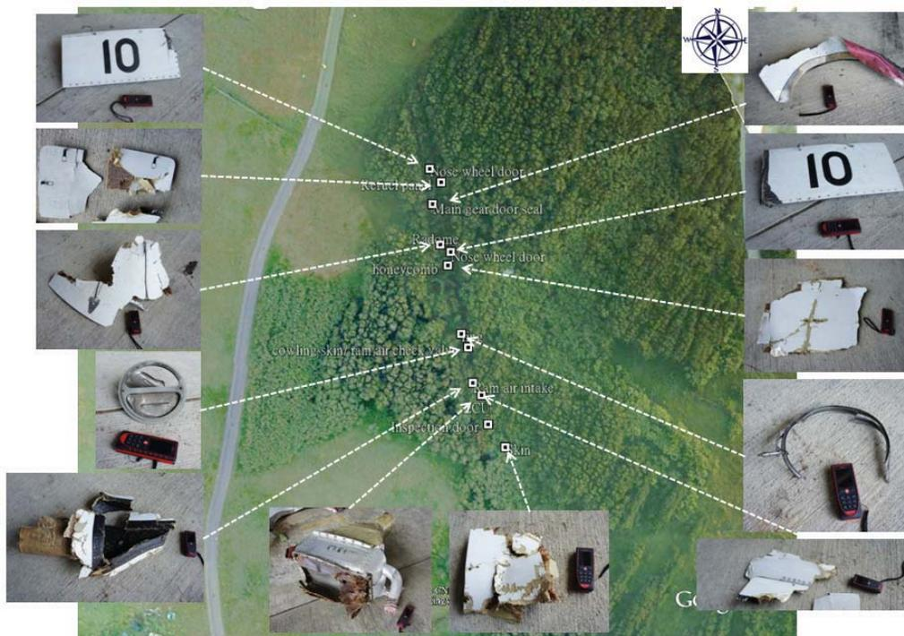
Figure 1.12-6 Superimposed aircraft wreckage distribution and component photos
