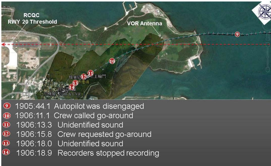
Figure 1.11-9 Superimposed GE222 flight path with satellite imagery for the last 40 seconds.
