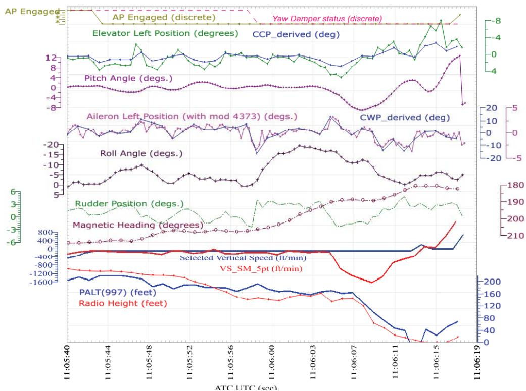
Figure 2.9-1 Relevant FDR and derived parameters
