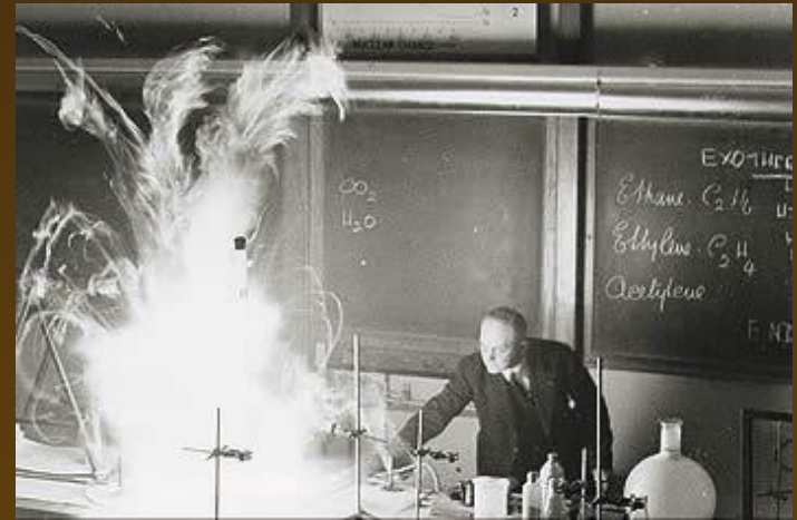
ignition of cotton wool soaked in liquid oxygen
