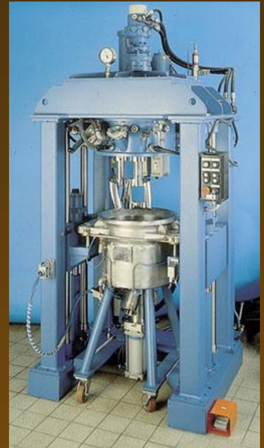
double-planetary mixer for fuel mixing
